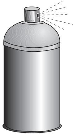
**Figure 1-3. Pressurized can sprayer. This common sprayer can be used to apply aerosol or liquid pesticides at high pressure.**
