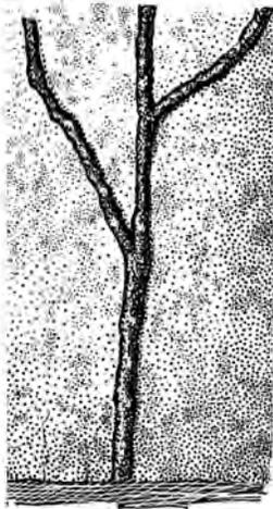
Figure 2-2. Subterranean termite shelter tube on a foundation wall. These protective tubes made of soil and fecal material are built across open areas and allow subterranean termites to leave the soil and infest wood above the ground.
