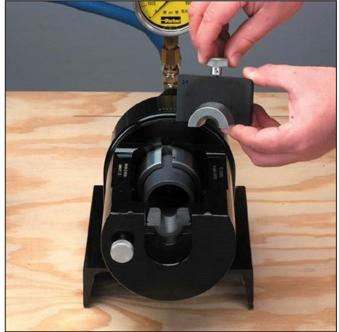
Step 7 Install Upper Die Install the Flaring Die half with the threaded hole into the upper half of the Die Retainer lower Die. Secure the die in place by turning the knurled thumb screw clockwise.
