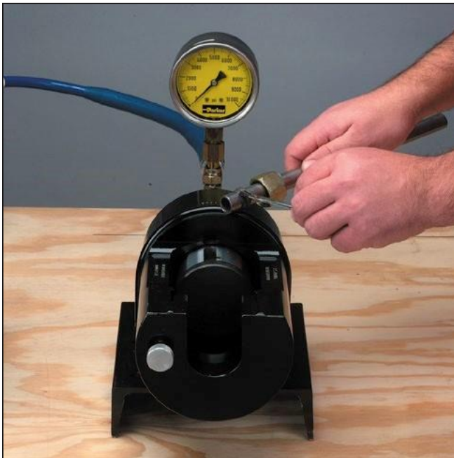
Step 6 Lubricate Ferrule Lubricate leading outer (bite) edge of ferrule with lubricant. Lubrication reduces wear on and reduces friction to ensure that all force is available to preset the ferrule.
