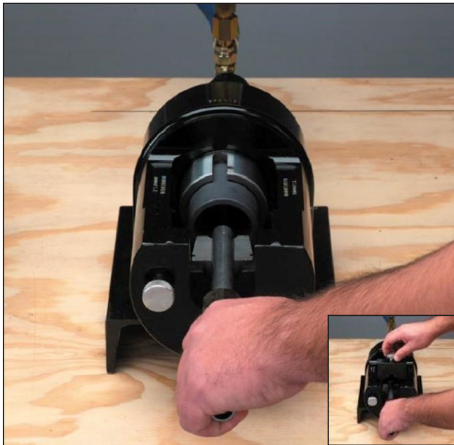
Step 8 Install Tube Place the properly prepared tube end to be flared on the lower die half in the HydraTool. Then, place the top Die Retainer with the Upper Die into the slot over the tube assembly.
