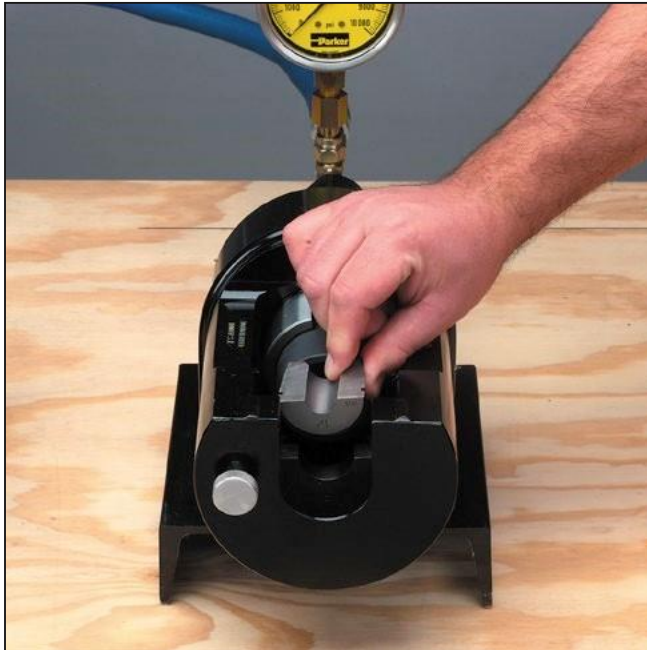
Step 6 Install Lower Die Halve Lubricate the outer conical surface of the Die half. Place the lower Die half in the Retainer. Assembly with the knurled thumb screw.
