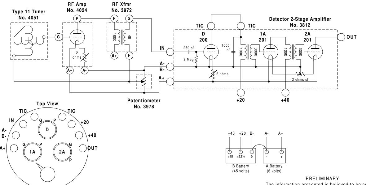
Note: This circuit is designed to use the type 200 & 201 tubes with 5 volt 1 amp filaments.
