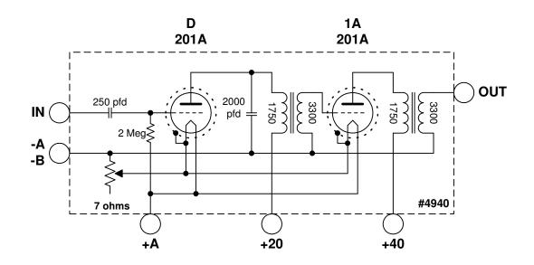
Note: This Detector / Amp is designed to use type 201A tubes with ½-amp filaments.
