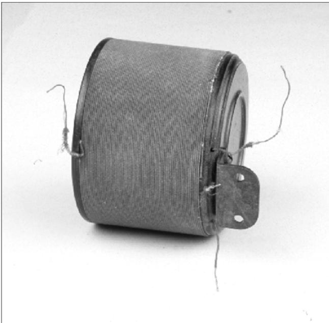
**Figure 3-21.** Type 6 RF transformer, bottom view.
