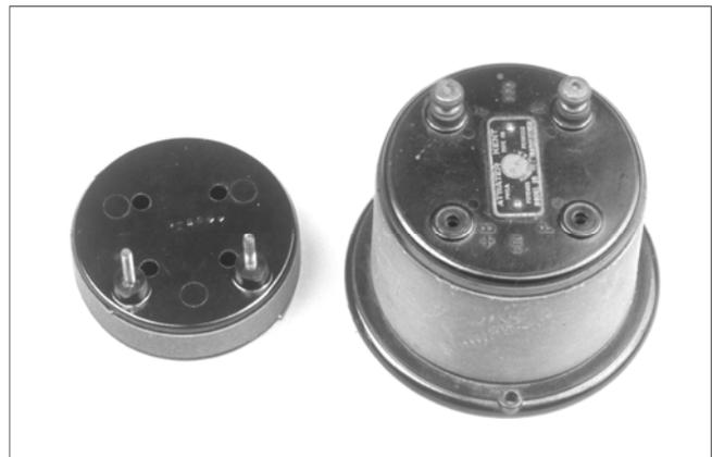
**Figure 3-7.** # 4326 RF transformer Type 1 disassembled, primary on the left. Note the un-drilled bosses on top near the terminals.
