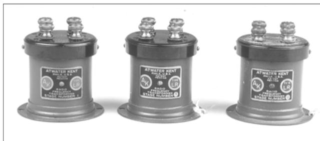
**Figure 3-4.** RF transformers: (Left to right) Stage 1 # 3802 late, Stage 1 # 3802 late, and Stage 2 # 3972.
