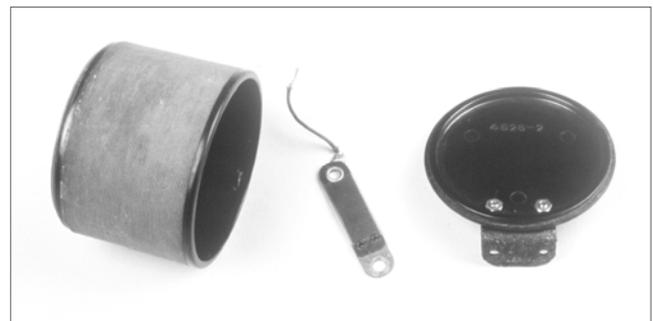
**Figure 3-23.** Type 6 RF transformer # 4946 disassembled, showing the grid resistor and end cap.
