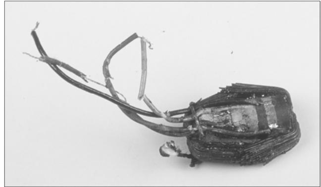
Figure 3-3. The uncased type L audio transformer # 3775.
