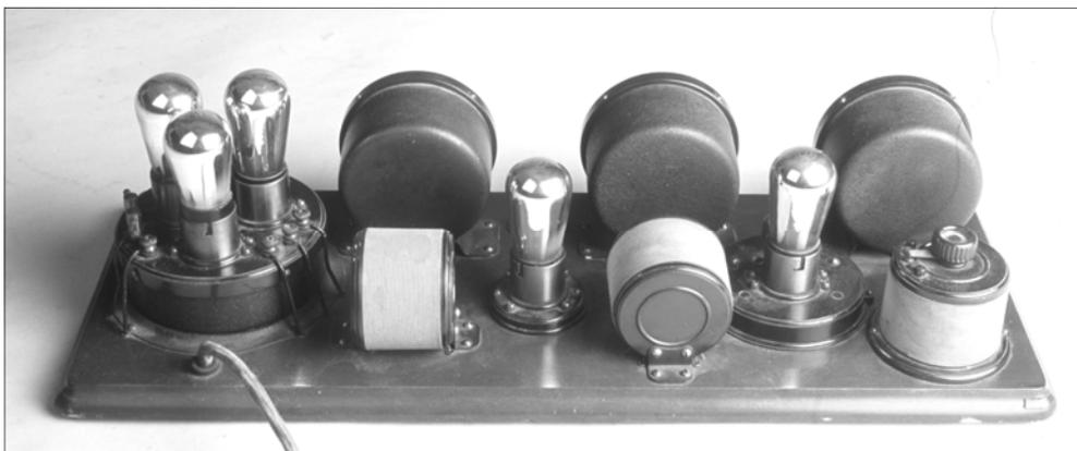
**Figure 3-15.** Model 10C #4700, rear view showing orthogonal transformers.
