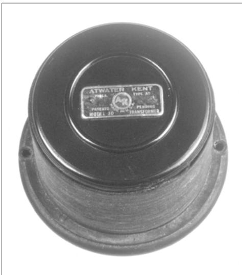
**Figure 3-13.** #4326 RF transformer Type 3 with raised ring.
