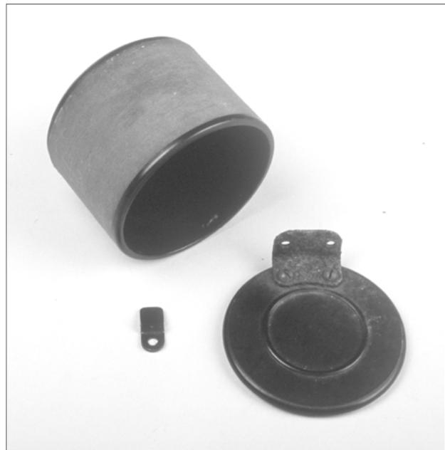
**Figure 3-19.** Typical 2<sup>nd</sup> or 3<sup>rd</sup> stage transformer with the mounting clip used on the B-suffix radios and the end cap used on the C-suffix radios.
