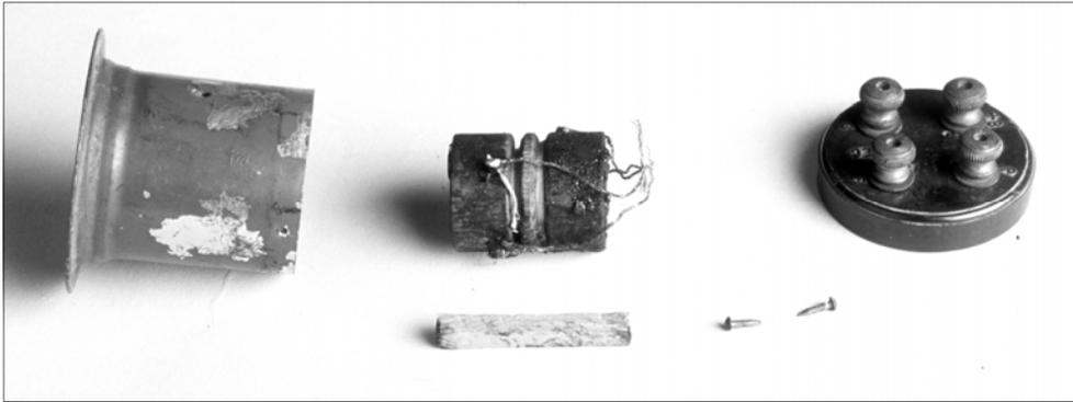
**Figure 3-5.** RF transformer # 3802 disassembled.
