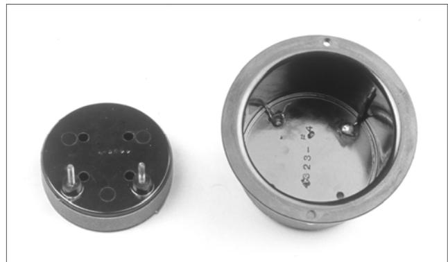
**Figure 3-8.** # 4326 RF transformer Type 1, bottom view, primary on the left.
