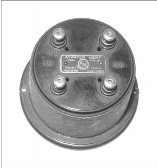
**Figure 3-9.** # 4326 RF transformer Type 2, as used on the Radiodyne # 4340 and Model 10.
