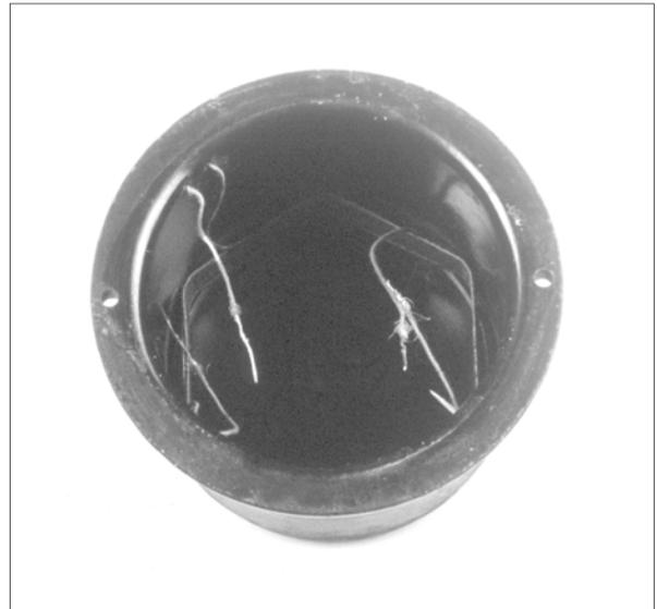
**Figure 3-14.** Detail of the primary coil in the Type 4 transformer.
