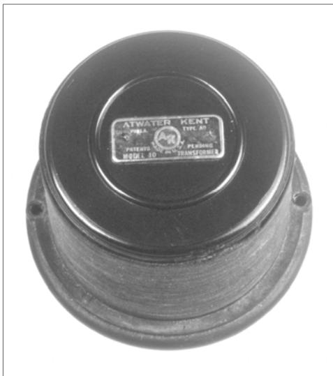
**Figure 3-13.** #4326 RF transformer Type 3 with raised ring.
