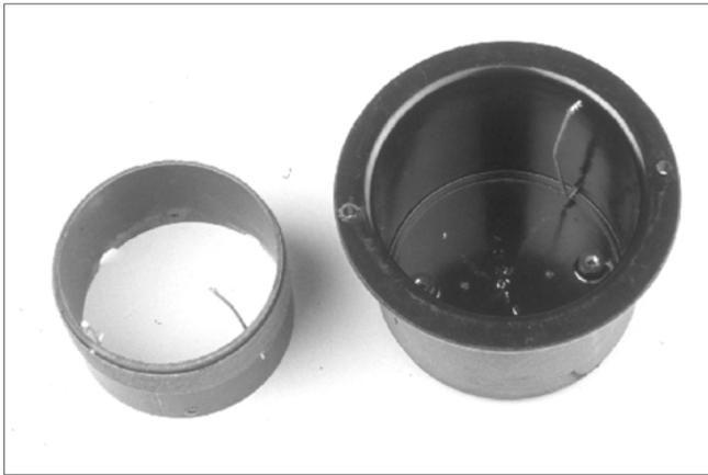
**Figure 3-12.** #4326 RF transformer Type 3 disassembled, underside view.
