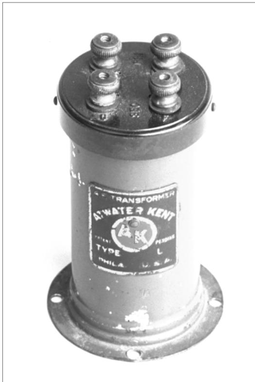
Figure 3-2. Type L audio transformer, # 3775.
