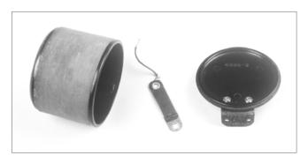
**Figure 3-23.** Type 6 RF transformer # 4946 disassembled, showing the grid resistor and end cap.
