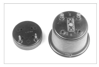
**Figure 3-7.** # 4326 RF transformer Type 1 disassembled, primary on the left. Note the un-drilled bosses on top near the terminals.
