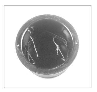
**Figure 3-14.** Detail of the primary coil in the Type 4 transformer.
