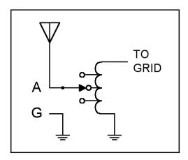
**Figure 3-16.** Schematic of antenna autotransformer connections for Types 5 and 6 transformers.
