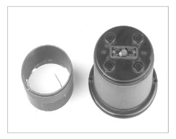
**Figure 3-11.** # 4326 RF transformer Type 3 disassembled, primary on the left.
