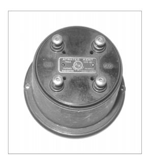
**Figure 3-9.** # 4326 RF transformer Type 2, as used on the Radiodyne # 4340 and Model 10.
