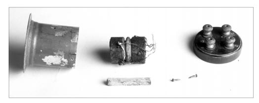
Figure 3-5. RF transformer # 3802 disassembled.
