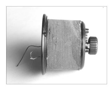
**Figure 3-17.** Type 6 RF transformer, #4633, showing the taps on the lower portion of the winding.
