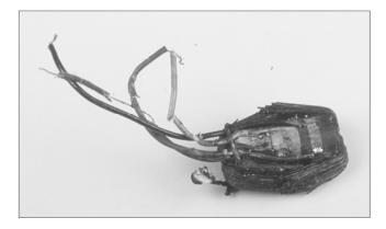
**Figure 3-3.** The uncased type L audio transformer # 3775.
