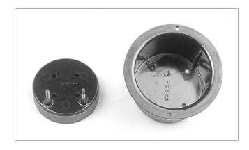
**Figure 3-8.** # 4326 RF transformer Type 1, bottom view, primary on the left.
