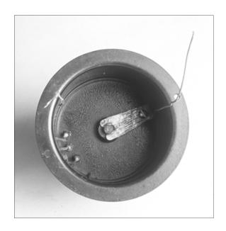
**Figure 3-18.** Type 6 RF transformer, #4633, internal view of switch configuration.
