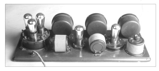
Figure 3-15. Model 10C #4700, rear view showing orthogonal transformers.
