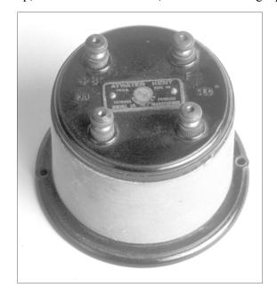
Figure 3-6. # 4326 RF transformer Type 1.
