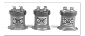
**Figure 3-4.** RF transformers: (Left to right) Stage 1 # 3802 late, Stage 1 # 3802 late, and Stage 2 # 3972.
