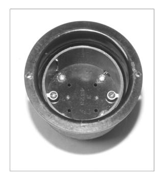
**Figure 3-10.** # 4326 RF transformer Type 2, underside view. Note wires soldered to screw terminals.
