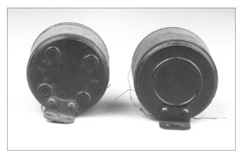
**Figure 3-20.** Type 6 RF transformers, 2<sup>nd</sup> and 3<sup>rd</sup> stages. Left: # 4636, 3<sup>rd</sup> RF in 10C and 12C, and # 4663, 2<sup>nd</sup> RF in 9C. Right: # 4946, 2<sup>nd</sup> RF in 10C and 12C.
