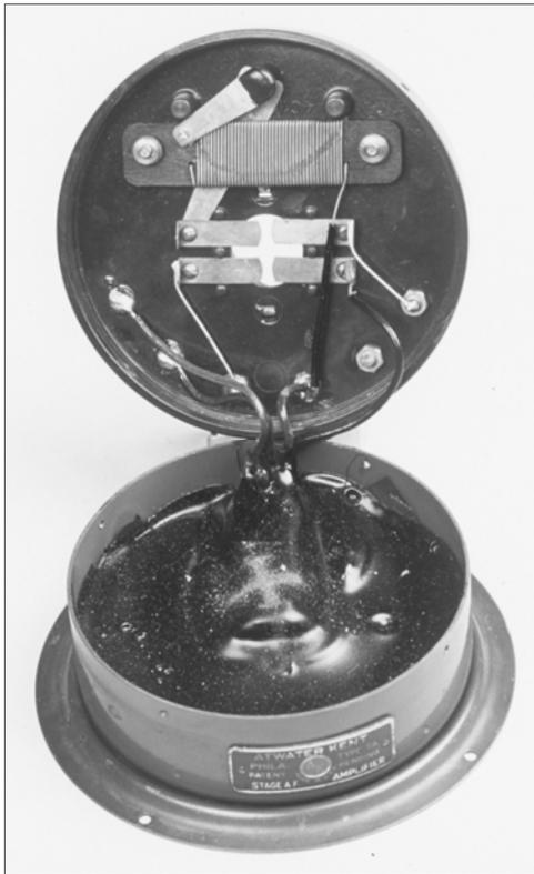
**Figure 6-2.** One-stage audio amplifier # 4030, interior view.
