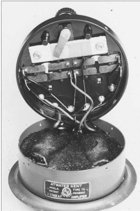
**Figure 6-4.** Two-stage audio amplifier # 3634, interior view.
