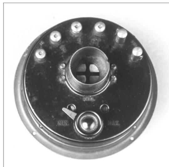
Figure 6-1. One-stage audio amplifier # 4030, top view.
