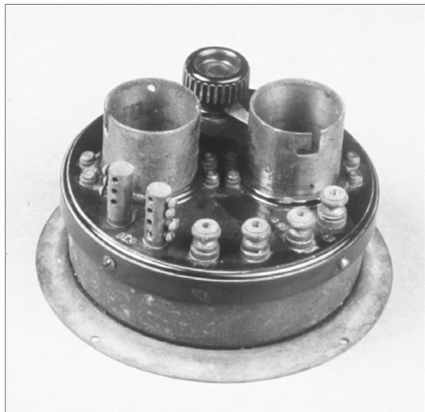
**Figure 6-6.** Two-stage audio amplifier # 3634, Type 2, rear view showing headphone posts.
