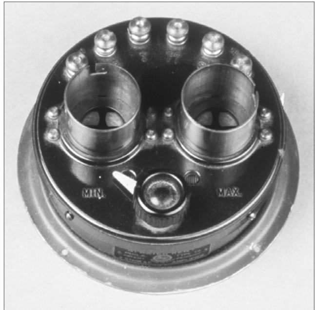
**Figure 6-3.** Two-stage audio amplifier # 3634 , Type 1, top view.
