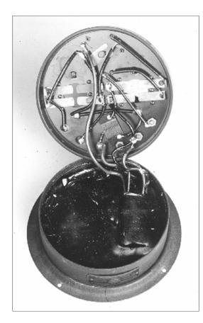
**Figure 6-16.** Two-stage audio amplifier # 4925, Type 7, interior view showing switch wiring and single audio transformer.
