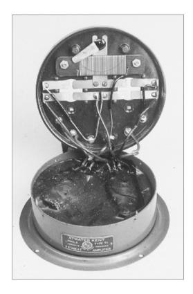
**Figure 6-8.** Two-stage audio amplifier # 3634, Type 3, showing 4-ohm fiber rheostat.
