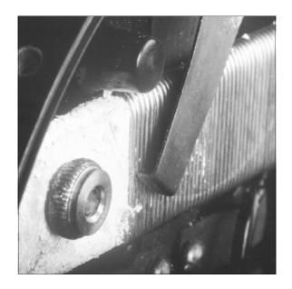
**Figure 6-5.** Two-stage audio amplifier # 3634 showing blunt-end rheostat slider and asbestos rheostat form.
