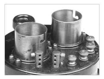
**Figure 6-10.** Two-stage audio amplifier # 3634, Type 5, rear view showing later headphone posts and tube key orientation.
