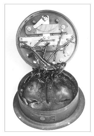
**Figure 6-11.** Two-stage audio amplifier # 3634, Type 5, interior view of TA used on the Model 12B # 4620 breadboard (typical of early and late versions).
