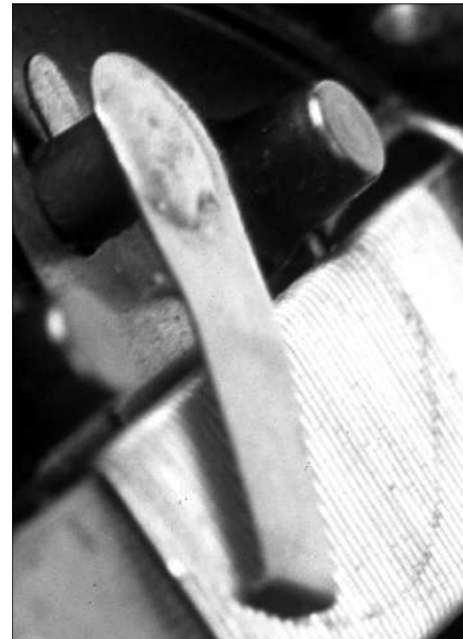
Figure 6B-4. Type 1 # 3676, detail of blunt-end rheostat slider.
