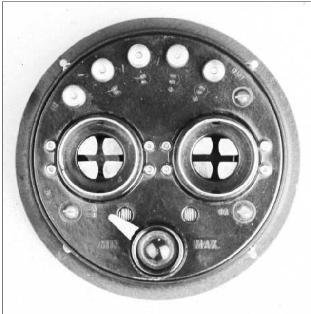
Figure 6B-12. Type 5 # 3676 (brown), top view (from early 12B # 4620). Note the P1-P2 labels at the upper left. The terminal labels do not indicate the actual function (see text).
