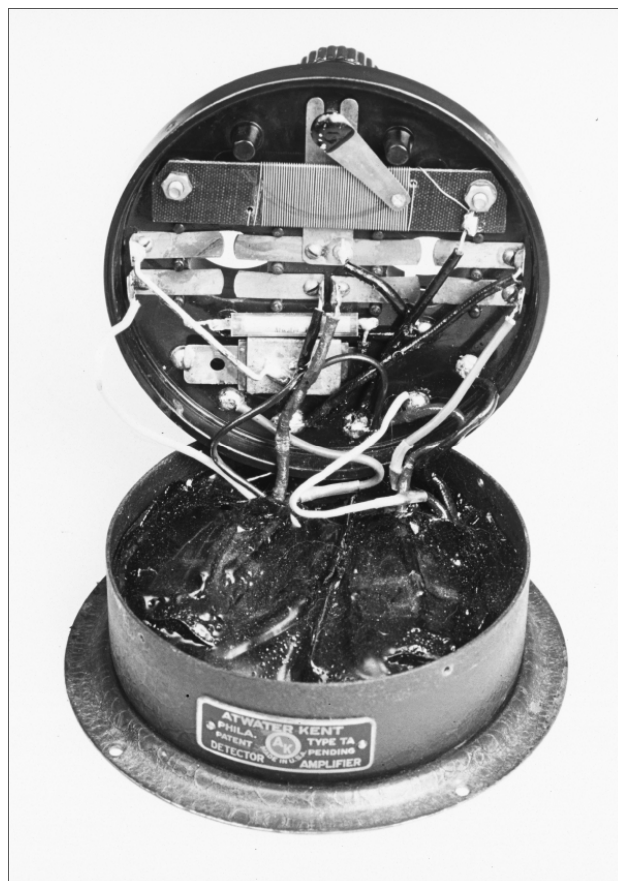
Figure 6B-18. Detector / Amplifier # 4940 (brown), internal view. Note the square bus bar wire used by the factory. Note also the first use of wire lug, on the right-hand rheostat screw.
