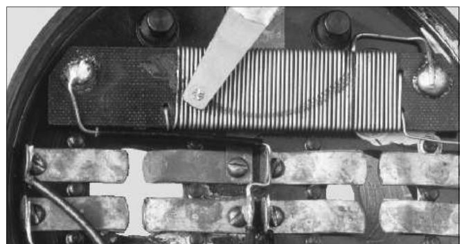
Figure 6B-8. Type 2 # 3676, wiring detail showing tapped rheostat winding.
