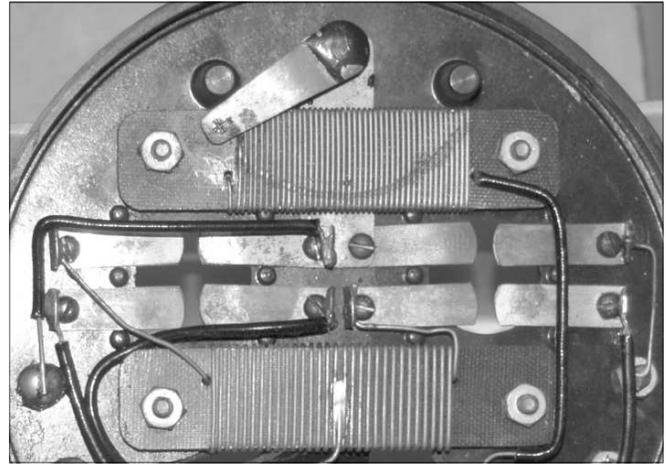
**Figure 6.** # 3812, Type 1 – filament resistors detail.
