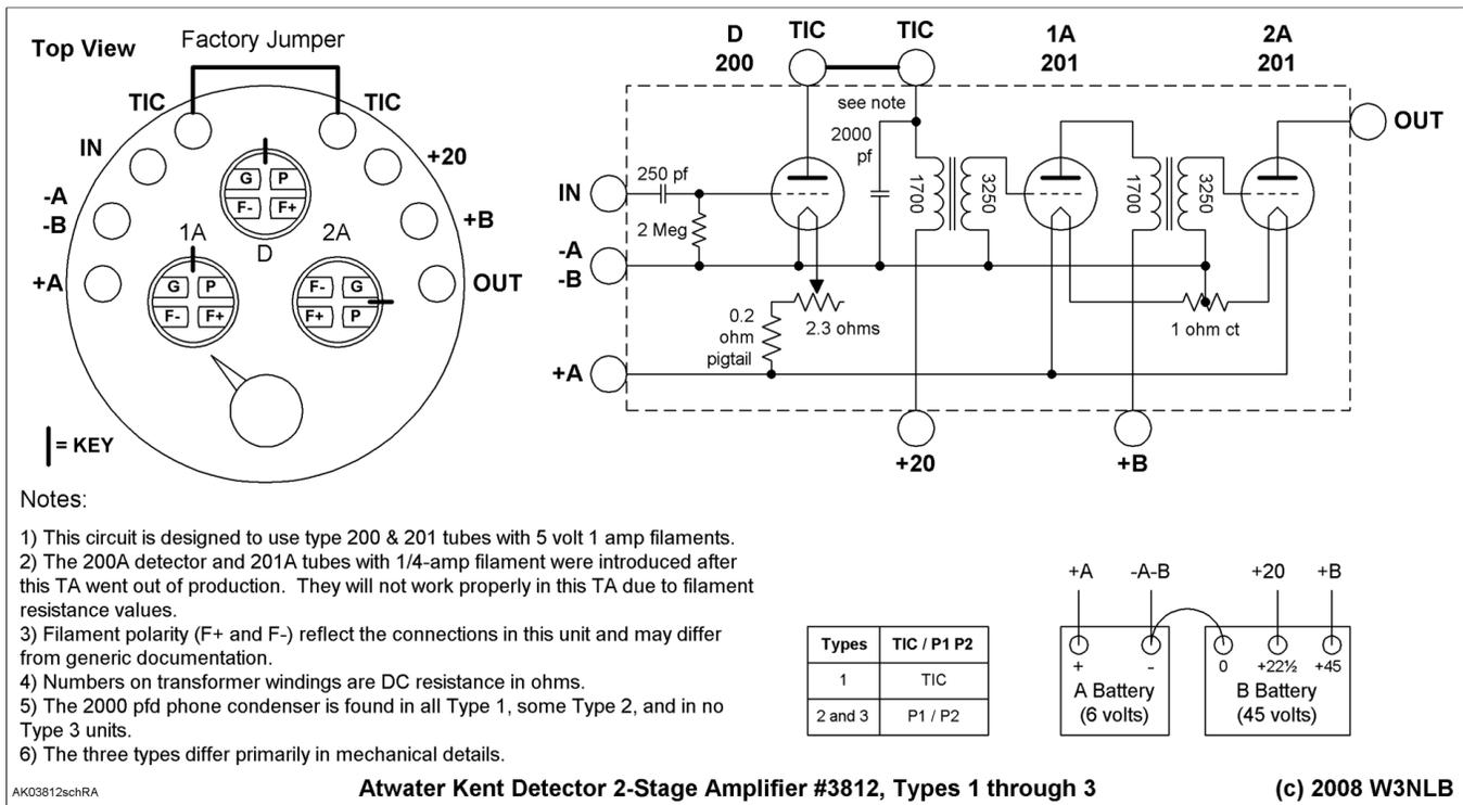
this # 3812 is that it does not have the 2000 pF phone condenser. All indications are that it was never installed at the factory, as opposed to being removed later during a service procedure. Apparently, starting with Type 2, some # 3812's were made with this condenser and some without.
