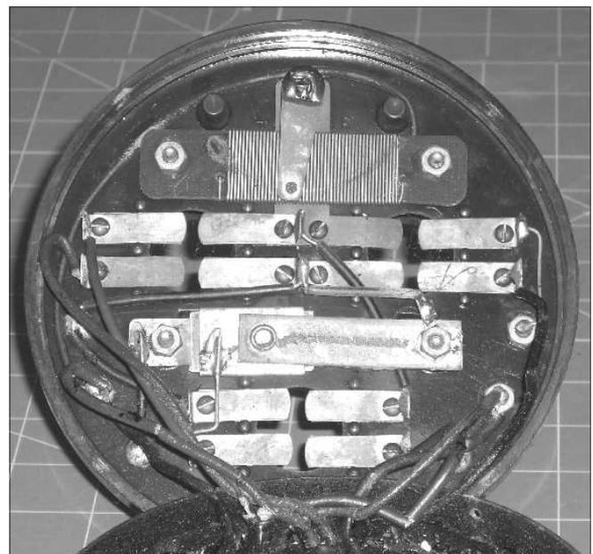
**Figure 19.** # 4520 – grid leak resistor to +A.
