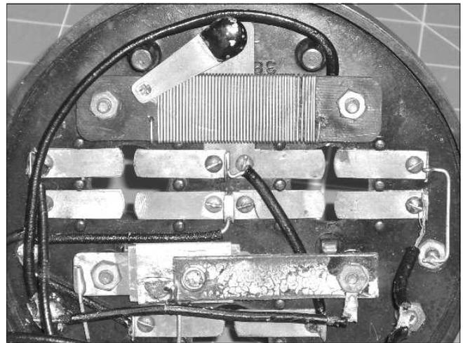
**Figure 18.** # 4520 – grid leak resistor to -A
