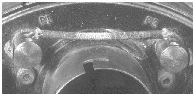
**Figure 9.** # 3812, Type 3 – P1, P2 two-hole terminal detail.
