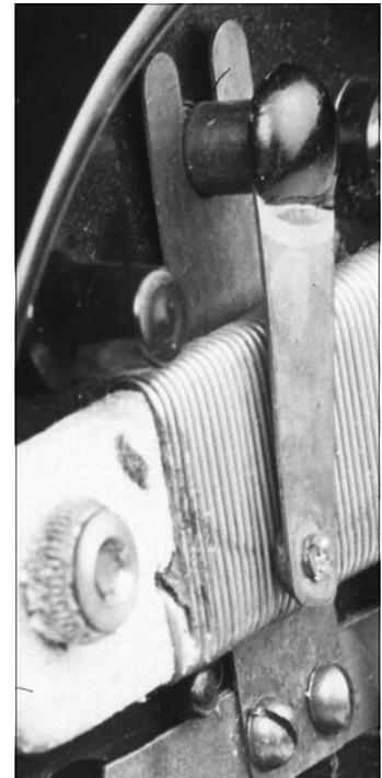
**Figure 7.** # 3812, Type 1 – filament rheostat contact detail.
