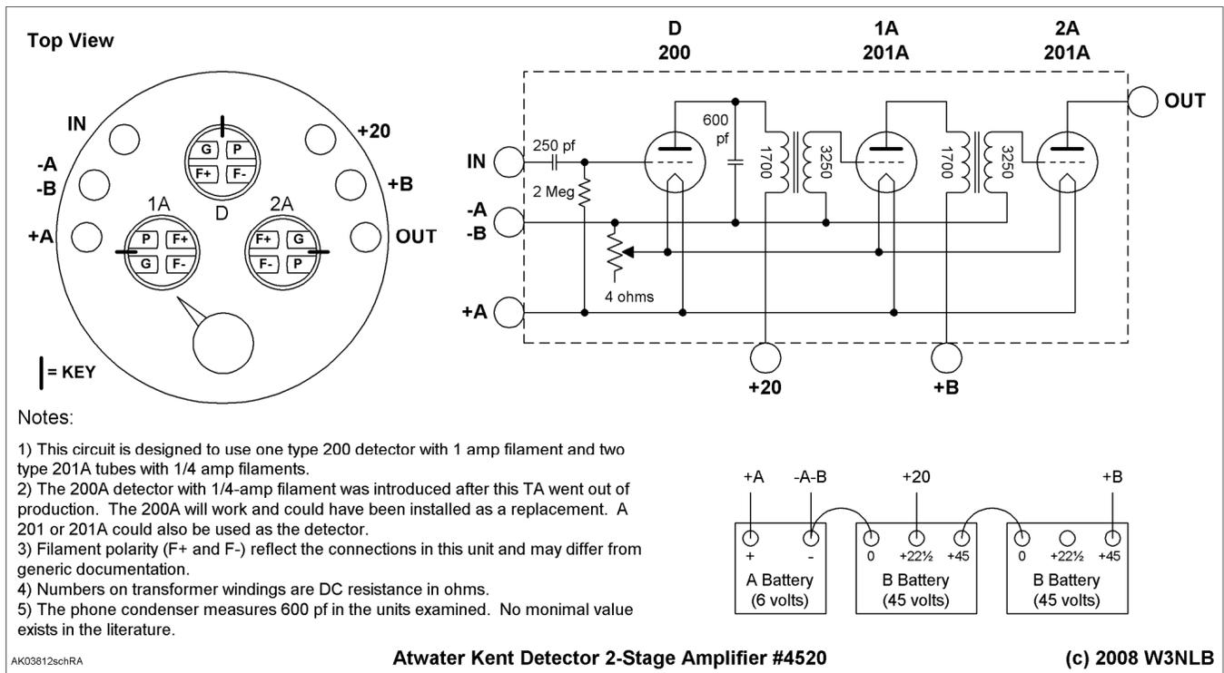
the output post lug to the plate pin on the audio output tube socket. The low side of the second audio transformer primary is connected to the solder lug on the **B+** post.
