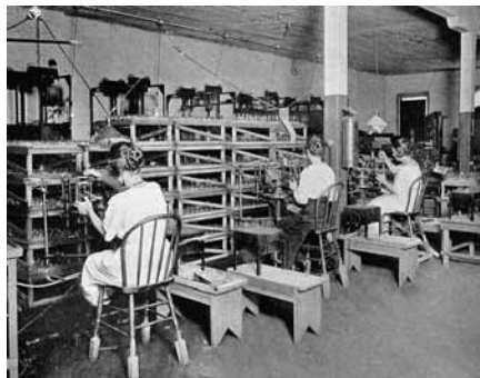
Fig.3. The Stem Manufacturing Dept. in the Moorhead Laboratories tube factory consisted of rudimentary production equipment with heavy reliance on manual labor. ( Moorhead and His Valve , Aug. 1919; courtesy of Stew Oliver)
