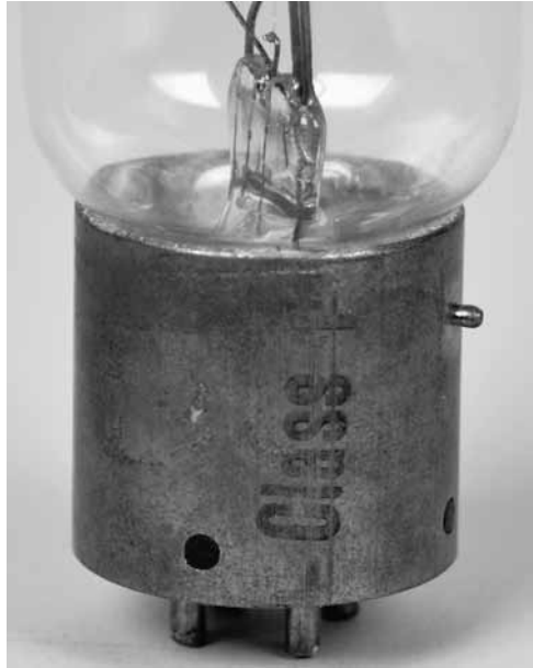
Fig.16. A small number of tubes with no letter stamped on the glass were rubber-stamped on the base with the appropriate class, such as this soft tube with the Class I stamp.
