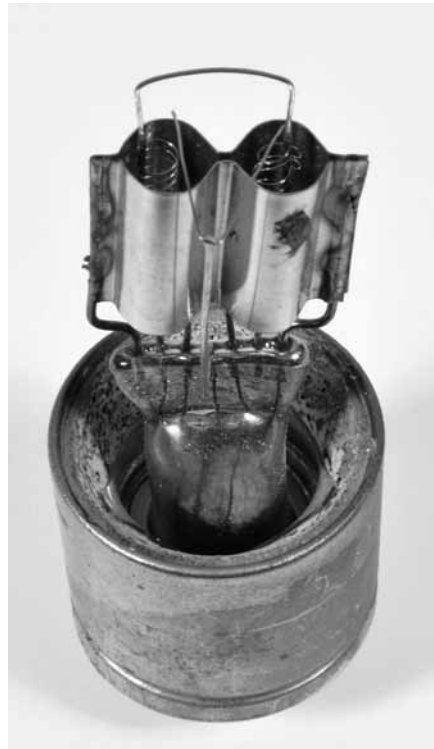
Fig.35. The Two-in-One tube consisted of two triodes enclosed within a single glass envelope (removed).
