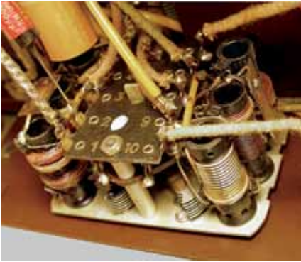
Fig.24. This particular model contains one of Geloso's extremely compact and efficient RF coil modules.
