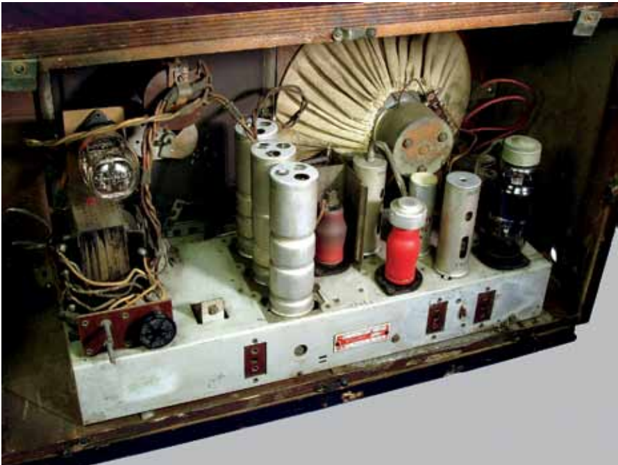
Fig.53. The R.F. coils were tuned on a semi-automatic fixture that rolled grooves into the aluminum can to the proper size. After this operation, it is impossible to remove the coils for repair.
