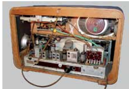
Fig.26. This Juwel 2 chassis is typical highly complex German design yielding performance rarely equaled by contemporary American radios.
