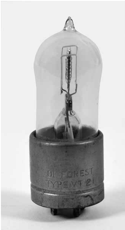
Fig.20. The mysterious “De Forest 20” tube appearing in the May issues of East Coast radio magazines may have referred to a soft version of this DeForest VT-21 manufactured for the U.S. Signal Corps during WWI.
