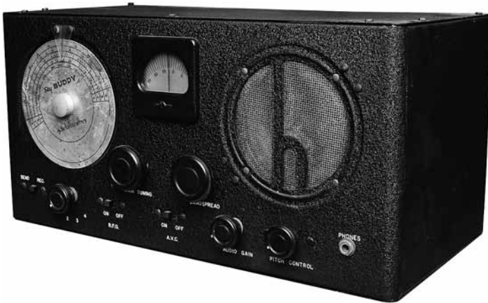
Fig. 10. Early Version of Hallicrafters S-19R Sky Buddy. All switches are slide type.
