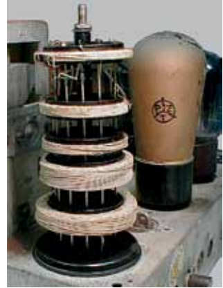
Fig.32. Note the PZT logo on the gold spray shield tube made by Philips in Poland.
