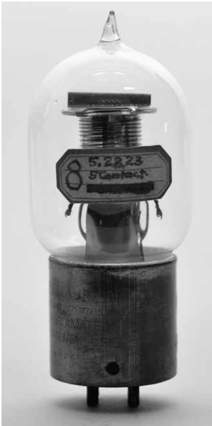
Fig.33. This Solenoid tube is one of forty prototypes tested by William W. Hanscomb between May and July 1923, each with a numbered sticker such as the one shown here with an 8 that corresponds to one of the forty different configurations numbered and documented in his laboratory notebook. (Stew Oliver collection)
