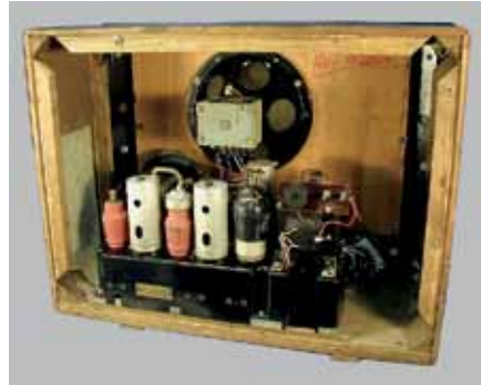
Fig.49. The chassis is a single robust Bakelite molding complete with tube sockets. The Speaker basket is also molded in Bakelite.
