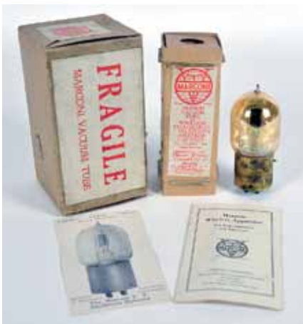
Fig.B7. Complete Marconi Tube Package: The egg-crate cartons containing the V.T. tubes were placed into a larger box for shipping along with a single “notice” sheet and a 12-page brochure with characteristic curves, a preferred detection circuit, and cautions for operating the tube.
