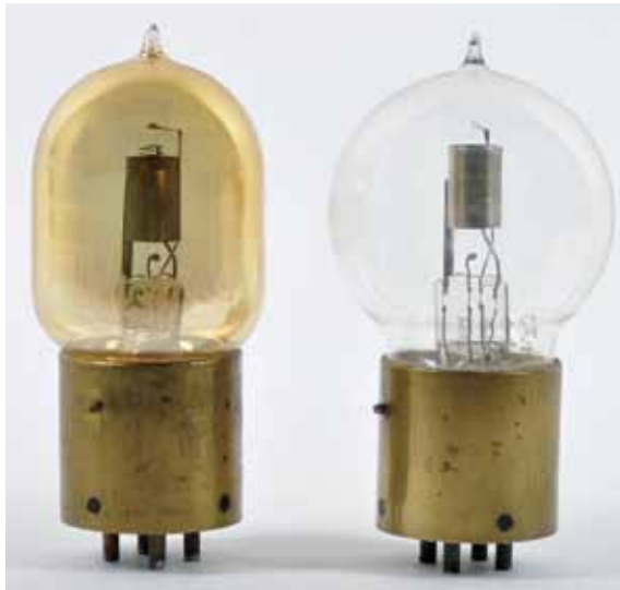
Fig.B4. Moorhead Postwar Tubes Sold by Marconi: The Moorhead hard A tube (left) and soft B tube (right) have the key physical characteristics of all Moorhead tubes sold by Marconi: either rounded cylindrical or spherical glass bulbs, either soft tubes with clear glass or hard tubes with or without a light-golden color getter coating, presses either with or without inking indicating tube type, and Shaw bases with or without the Marconi globe logo, DeForest name and patent information.
