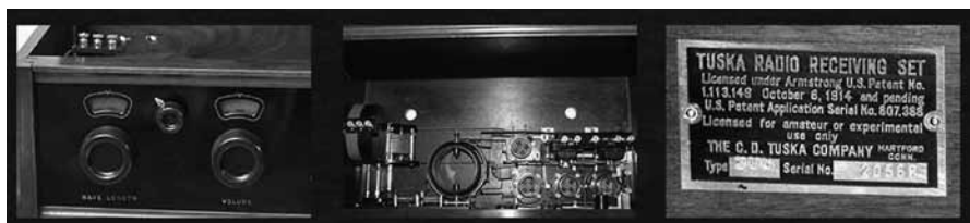
Fig.9. A triptych of the Superdyne with details of Tuska’s patent application no. 807,388 at the right. From the Steve Johannessen (AWA) collection, his photo. This appears to be a model 305. Radiomuseum.org notes additional Superdyne models. 228, 301, & Superdyne Jr., and there may have been other models.
