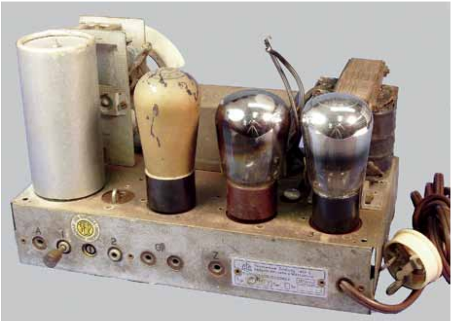
Fig.33. A single tunable antenna notch filter is mounted to the back wall of the chassis. Note the mains plug, a design used in Australia since 1937.
