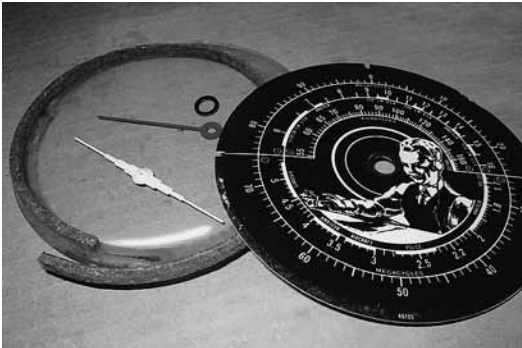
Fig. 7. Parts of the 5-T With Boy: dial, dial glass, seal, celluloid dial, red pointer, washer and beige press-on pointer. The 5-T Without Boy has a similar dial with slightly different calibration, a larger hole in the red pointer and a beige pointer held in place with a screw.
