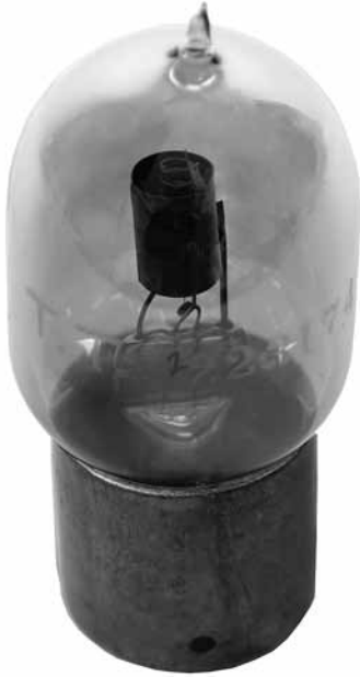
Fig.27. While this transmitting tube was stamped with T.T. on the glass, the numeral 2 inked on the press and the serial number of 223,174 stamped on the bulb indicate that it is most likely an ordinary V.T. tube with a higher than normal vacuum.
