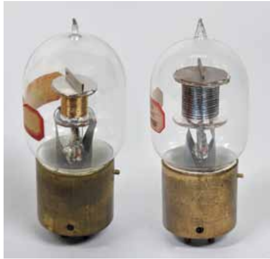
Fig.B18. Prototype Solenoid Tubes: These two tubes with red labels identified by the numbers 7 and 8 (left to right) are two of forty different prototype solenoid tubes identified by number in the laboratory notebook of consultant William W. Hanscomb, who tested the tubes under the auspices of Atlantic-Pacific Sales Co. between May and July of 1923; note the difference in solenoid coil dimensions and material. (Joe Knight and Stew Oliver collections)
