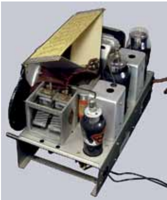
Fig.20. The 6AY8 duodiode – beam power tube in this receiver was never used in the USA. It is equivalent to the side contact EBL1.
