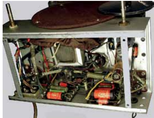
Fig.21. Most small components mounted on 'tag boards'. Note cloth bag over speaker to keep voice coil free of contamination.
