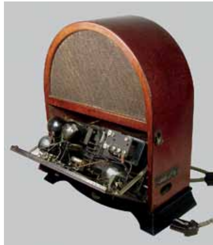
Fig.44. Electrical standards of the day required that the mains be disconnected if the cabinet were open.
