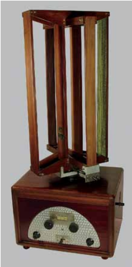
Fig.12. A combination loop antenna for Long Wave and Medium Wave reception.
