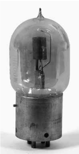
Fig.5. All of the tubes manufactured by Moorhead for sale by Marconi were derivatives of the SE-1444 developed for the Navy during the war.
