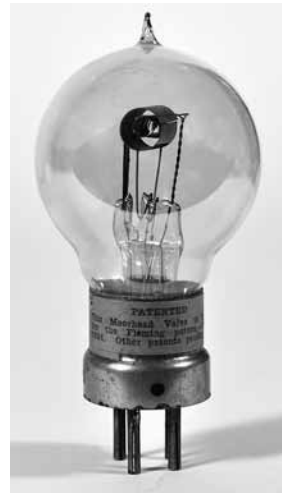
Fig.7. Moorhead manufactured the British Type B transmitting tube, which was similar to the Type R tube but with a horizontal plate that had a grid of 22 turns—twice the number used in the Type R. (Stew Oliver Collection)
