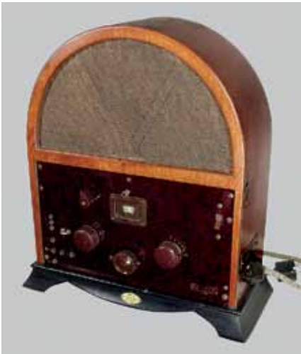
Fig.43. This NORA K3Wf represents the first series of German table radios to have a built-in speaker and are mains powered.
