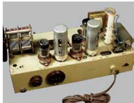
Fig.42. The I.F. transformers have octal tube socket bases that plug into the chassis. How was this cost effective?
