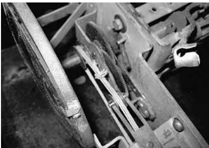
Fig. 5. Close up of the 5-T With Boy Sky Buddy tuning mechanism showing handmade string belt to replace the original belt. Also shown is the idler/tensioner under the string belt. Such string belts were used mainly to avoid the complex disassembly needed to replace the proper belt. Also shown is a soldered-on tab to replace one damaged in the past.
