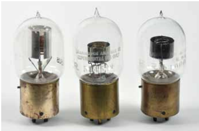
Fig. B13. Soft E.R. Tubes: Soft E.R. detector tubes with Shaw bases introduced by Moorhead Labs in mid-1920 evolved from the prewar unbased Electron Relay; the earliest version had a spiral copper grid and a cylindrical aluminum plate with tabs extending down and bent against the press and (left), while later versions had a nickel grid and plate half the height of the earlier plate—one version of which was shiny (middle) and the other was black (right).
