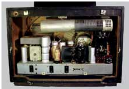
Fig.55. RF coils like the MAS-24 but Philips uses the more familiar type of tuning capacitor. Note the cylindrical module suspended from the top of the cabinet.
