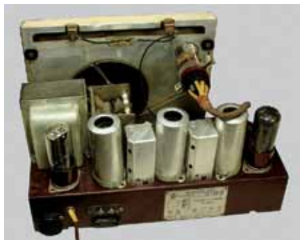
Fig.23. High quality Geloso components such as tuning capacitors, I.F. coils and tube shields were used by other manufacturers.
