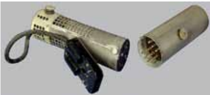
Fig.56. Optional DC Mains converter. You choose one of two DC mains input modules that plug into a vibrator circuit that outputs 220 VAC to power the radio in the usual way.
