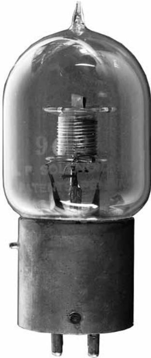
Fig.34. This tube with serial number 962, A-P Solenoid and Patents Pending stamped on the glass was one of approximately 2000 production tubes sold by A-P Laboratories. (Joe Knight collection)
