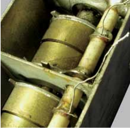
Fig.52. Three sets of high precision brass spirals mesh to tune the receiver.
