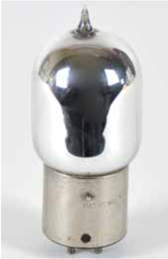
Fig.B17. Moorhead Prototype with Rectangular Plate: This unusual triode tube with a nickel base marked "PAT PEND" is believed to be a Moorhead prototype with an upright rectangular plate structure open only at the top and bottom but not on the sides, a configuration that suggests it may have been intended to be a power amplifier tube made circa 1920.
