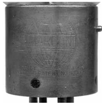
Fig.39. The Shaw brass base characterized in the text as a “D/M base” had the Marconi globe logo and Fleming patent number shown here stamped on one side, and the DeForest name and patent information stamped on the opposite side.
