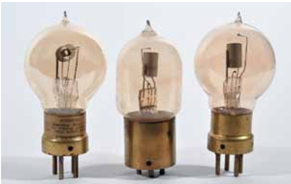
Fig.B2. Moorhead Wartime Tubes: During WWI Moorhead manufactured three tubes in quantity, the British Type B transmitting valve (left), the British Type R receiving valve (right), and the SE-1444 receiving audion for the U. S. Navy with a Shaw base (center). (Stew Oliver and author’s collections)
