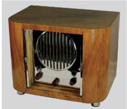
Figs.15 & 16. Modernist cabinet design – Chrome plated face plate behind translucent celluloid sliding doors.
