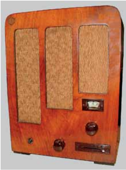
Fig.30. This ECHO model PZT-121-Z is essentially electrically equivalent to the German VE-301 Peoples Radio.
