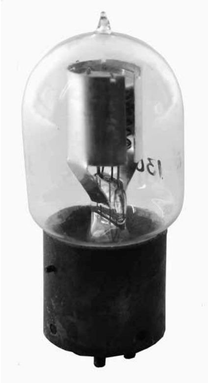
Fig.24. The earlier postwar E.R. tubes had a tall cylindrical plate similar to the prewar unbased tubular Electron Relay but with a support consisting of tabs bent down against the press, tabs which do not appear in postwar ads or brochures (the version shown here also has a mica spacer at the top).
