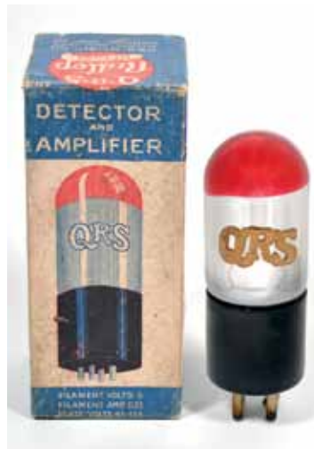
Fig.B22: Q R S Redtop Tube with Carton: A Q R S Redtop tube with two triodes in a single envelope similar to the Two-in-One tube was manufactured by the Q R S Music company circa 1925-6 using equipment it purchased from the defunct A-P Laboratories. (Sunny Clutter collection)
