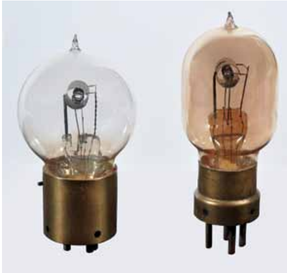
Fig.B3. Moorhead British Type B Variants: Two variants of the British Type B manufactured by Moorhead are the Type B with a Shaw base believed to be a prototype made in small quantities (left), and the Type VT-32 with a tubular bulb made in quantity during and/or after the war (right). (Stew Oliver collection)
