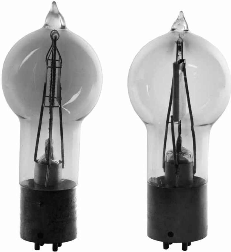
Fig.29. The A-P Rectifier tube appearing in A-P ads looked more like the DeForest Singer Power Triode with a Shaw base (left) than the actual A-P Rectifier tube (right). (Stew Oliver and E. Wenaas collections)
