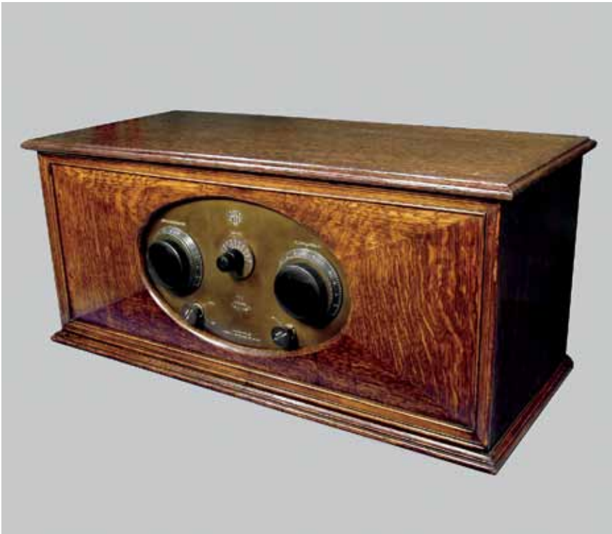
Fig.9. The cabinet is ‘flaky cut’ oak and the grain is filled but not leveled; somewhat in the style of the Victorian era Jacobean furniture revival.
