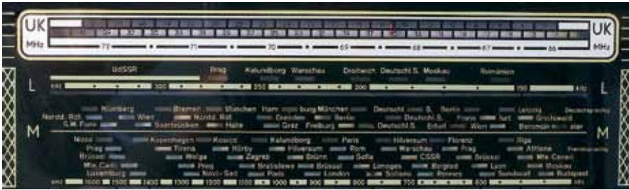
Fig.27. The ‘Stationized’ linear dial so very common in European radios showing a FM band tuning the Eastern Bloc frequency range of 65 to 74 MHz.
