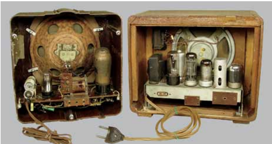
Figs. 46 & 47. At left is the pre-war set similar to the DKE-38. On the right is the Communist era 'channelized' receiver.
