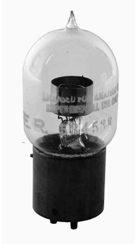
Fig.25. E.R. tubes with serial numbers greater than ~511,000 had a cylindrical plate about half the height of earlier E.R. tubes.
