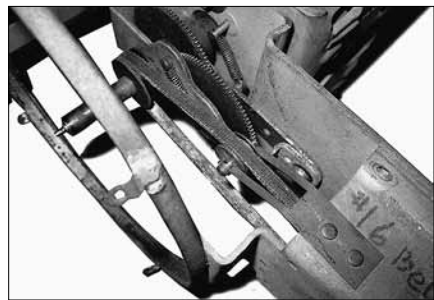
Fig. 6. Properly installed General Cement No. 116 Belt in a 5-T With Boy Chassis. Note glass, dial and hands have been removed and the soldered tabs bent out to facilitate removal of these parts. One of the tabs had broken in the past and was replaced.
