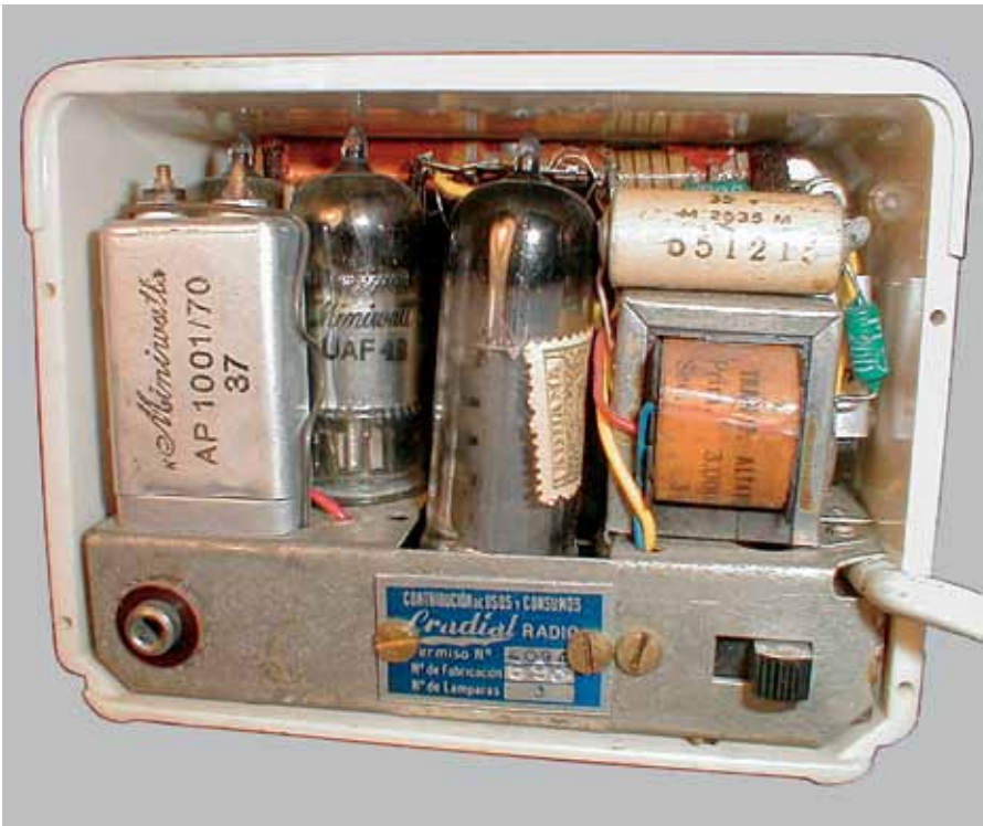
Fig.6. Tubes stay in place simply because there is only about 1.5 mm clearance to the top of the cabinet. (Back safety cover removed.)
