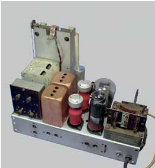
Fig.29. The brown faced box on the left side of the chassis contains two tunable antenna notch filters (one for LW & one for MW) to prevent overloading the high gain tuned RF stage of this radio.
