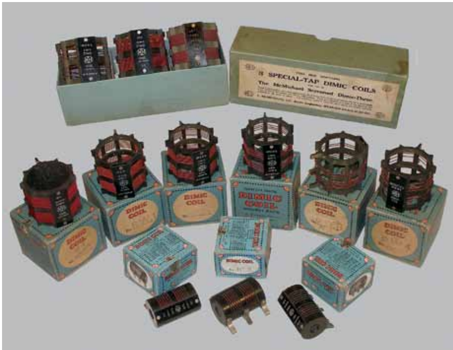
Fig.11. 3 standard coils were supplied with the receiver. There were 9 other optional coils available.
