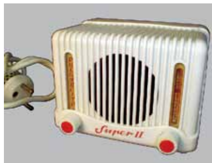
Fig.4. Tiny cabinet has no room for a tube filament voltage dropping resistor. This resistor is built into the oversize mains plug.
