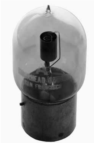
Fig.13. This Class II tube with a serial number 93 was stamped with the letter A and Moorhead Laboratories followed by San Francisco on the glass envelope.
