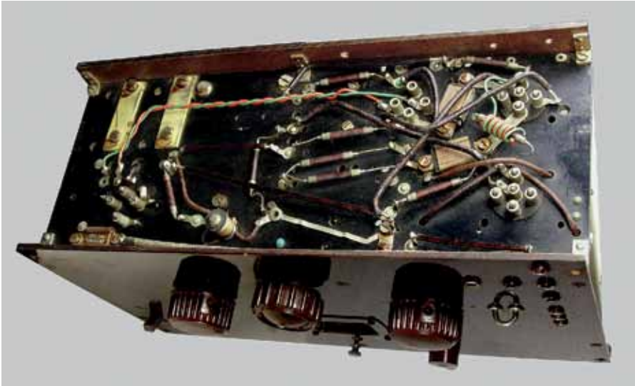
Fig.45. German manufacturers were the first to develop high stability high value resistors that remain within tolerance even after 80+ years.
