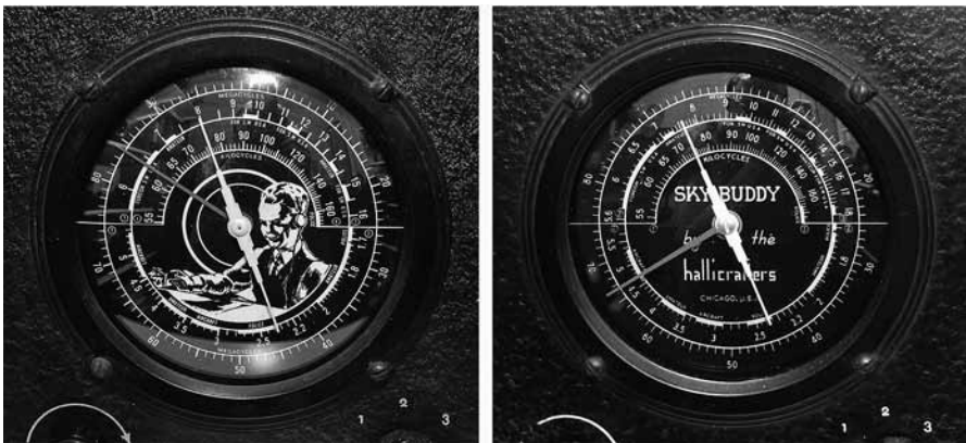
Fig. 4. Comparison of the 5-T Celluloid Dial With Boy and the one Without Boy showing on the dial. "SKY-BUDDY by The Hallicrafters". See back cover for color. The small red pointer is the 36 to 1 bandspread dial for the 0-100 outer ring of the dial. The longer beige colored pointer is to show frequency, the upper pointer for Band 1 and 3, the lower portion for Band 2.
