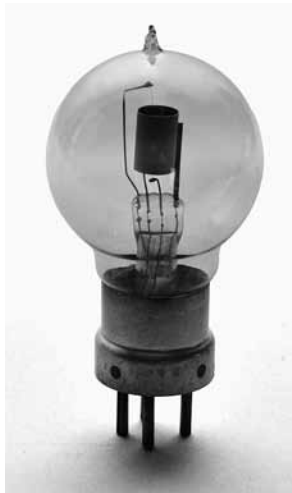
Fig.6. The British government contracted with Moorhead during the war to manufacture this Type R receiving tube, which was fashioned after the French Type TM valve but with a vertical plate structure. (Joe Knight collection)
