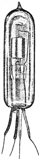
Fig.9. Moorhead prepared a price sheet circa March 1919 to advertise four vacuum valves designated Relay for detection/amplification/oscillation, Type R for reception, Type RH as an oscillator and amplifier, and Type B for transmitting—described as being exactly the same as that being furnished to the U.S. Navy. (Courtesy Stew Oliver)
