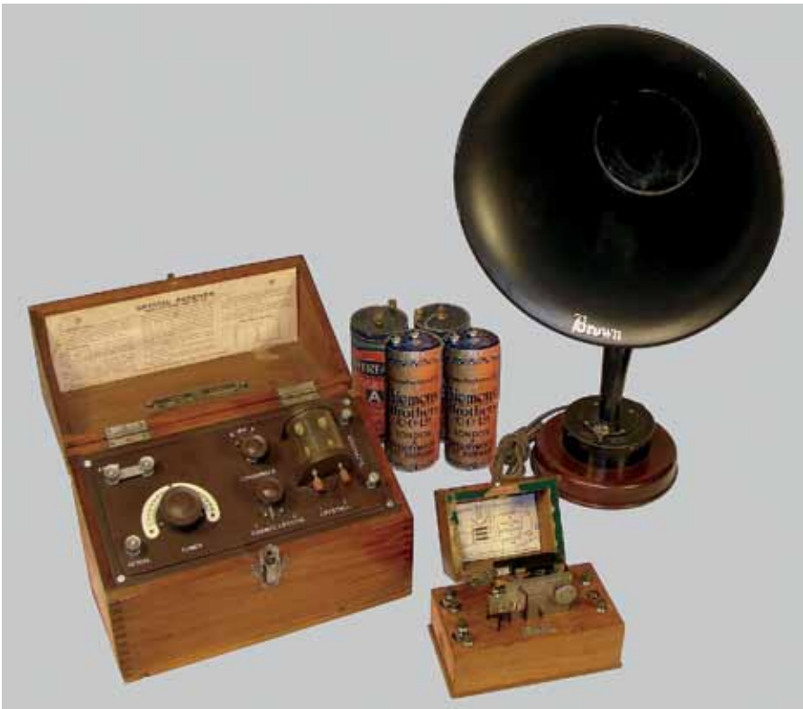
Fig.7. B.T-H Crystal Set with S.G. Brown Microphone Amplifier & Horn speaker. Powered by 6 Volt dry cell battery.
