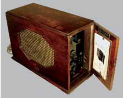
Fig.34. Controls mounted on the side of the cabinet concealed by a door. Instruction manual fits under clips mounted to the door.
