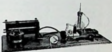
THREE SLIDE COIL RADIOSON ELECTROLYTIC DETECTOR, WITH PLUNGER BATTERY.
