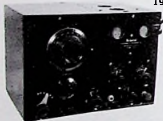
FEDERAL 57 RECEIVER SINGLE TUNED RECEIVER 1 STAGE R.F. DET. 2 STAGE AUDIO 1922 S.P. $98.00
