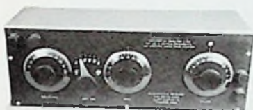
CLAPP-EASTHAM ZRF REGENERATIVE TUNER 2 VARIOMETERS 1 VARIOCOPLER 1919 $38.00
