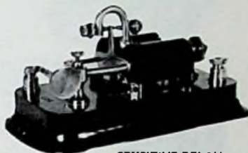
SENSITIVE RELAY USED WITH COHERER DET. 1910
