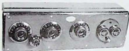
ATWATER KENT MODEL 20 C COMPACT 5 TUBE TRF 1925 $80.00 ("BIG BOX" MODEL 20 WAS ANNOUNCED IN 1924)
