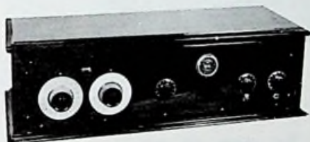
REMLER 9 TUBE SUPER 45 KC. IFs 1925 KIT $90.00
