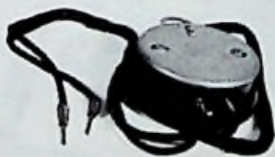
SAMPSON WATCH CASE RECEIVER HAND MADE PHONE TIPS ABOUT 1912
