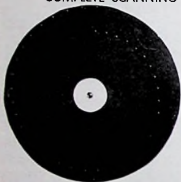
36-aperture scanning disc
