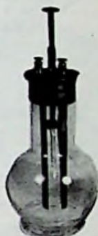
BICHROMATE BATTERY PLUNGER TYPE ABOUT 1900
