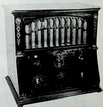
RADIOLA X REGENOFLEX 4 WD 11 TUBES 1925 S.P. $245.00
