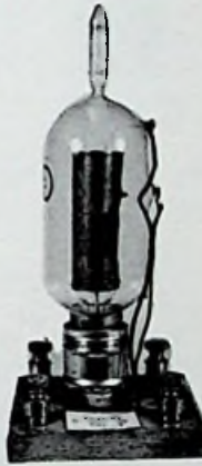
MARCONI TUBE MADE BY H. J. ROUND 1911
