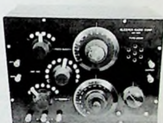
SLEEPER TYPE 3300 REGENERATIVE RECEIVER 1920 $35.00
