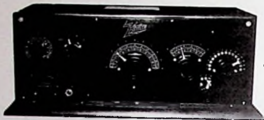
ZENITH 4R REGENERATIVE RECEIVER 1923 4 TUBES $100.00
