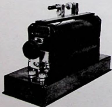
AMRAD TYPE C SPARK INDUCTION COIL MADE FOR U. S. ARMY IN 1918.
