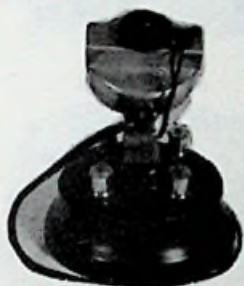
AMPLIFIER FOR CRYSTAL SET CARBON MIKE DIRECT COUPLED TO A RECEIVER. OPERATES A LOUDSPEAKER WITHOUT TUBES.
