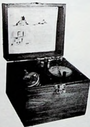
RADIOLA SIX TUBE RECEIVER WITH RE-ANT TUNER. AR-THREE STAGE R.F. AMP. RA-REGEN RECEIVER. DA-DET TWO STEP AMP. MADE BY WESTINGHOUSE 1922 S.P. $225.00
