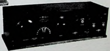
GREBE CR-9 THREE TUBE REGEN. 150 TO 3,000 M. 1921 $110.00
