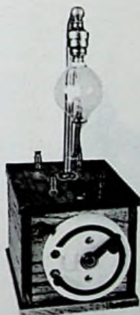
AUDION CONTROL BOX FOR DEFOREST AUDION 1910
