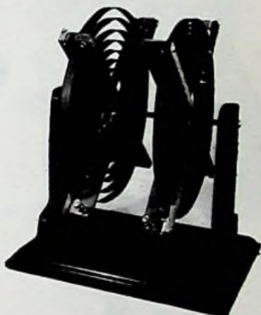
AMCO OSC. TRANS. 1 KW MADE FROM KIT ABOUT 1914
