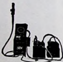
This is the way "B" Storage Batteries are charged with Tungar and attachment.
