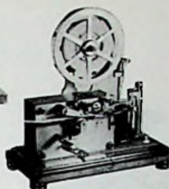
BRANLEY COHERER AND DECOHERER WITH KEY WIND TAPE PRINTER ABOUT 1902 TO 1905
