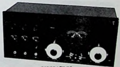
RADIOCRAFT D6 REGENERATIVE 1923 3 TUBES
