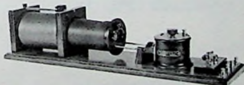
THREE CIRCUIT LOOSE COUPLER RECEIVER FOR CRYSTAL DETECTOR OR AUDION. 1919
