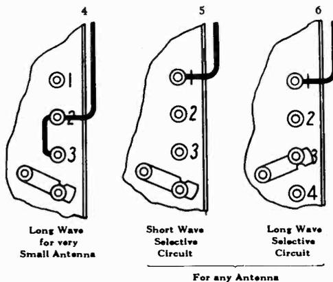
Fig. 3—Showing Antenna Connections to Different Binding Posts
