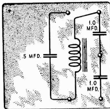
Figure 8—Internal connections of condensers.
