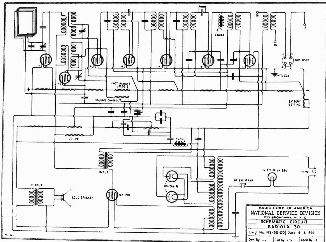
Figure 13—Schematic circuit diagram of Radiola 30
