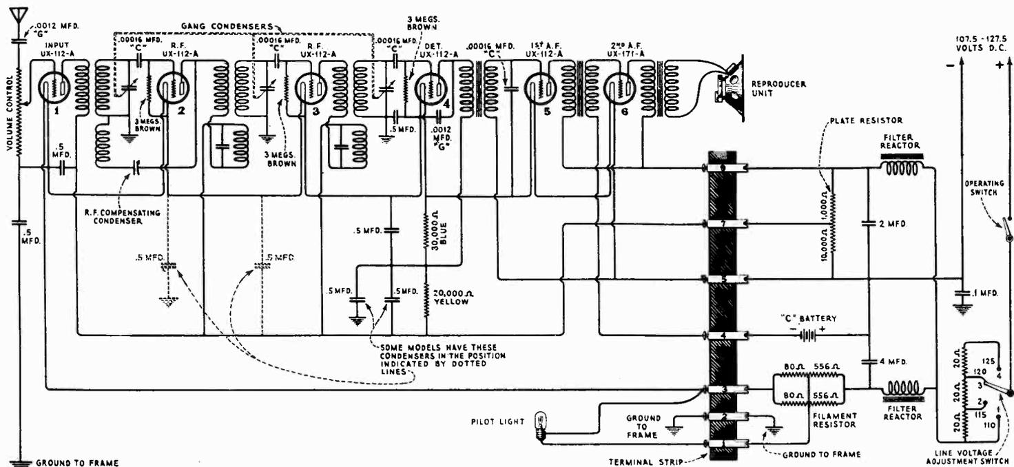
Figure 5—Schematic circuit diagram of Radiola 51 D.C.
