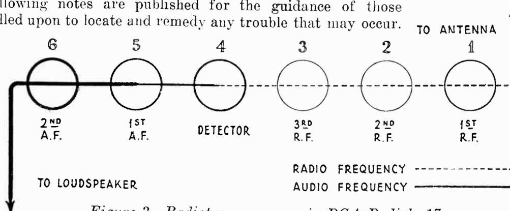
Figure 3—Radiotron sequence in RCA Radiola 17
