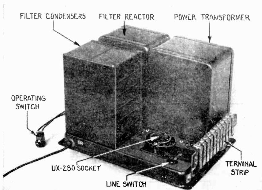
Figure 2—Socket Power Unit showing various parts.
