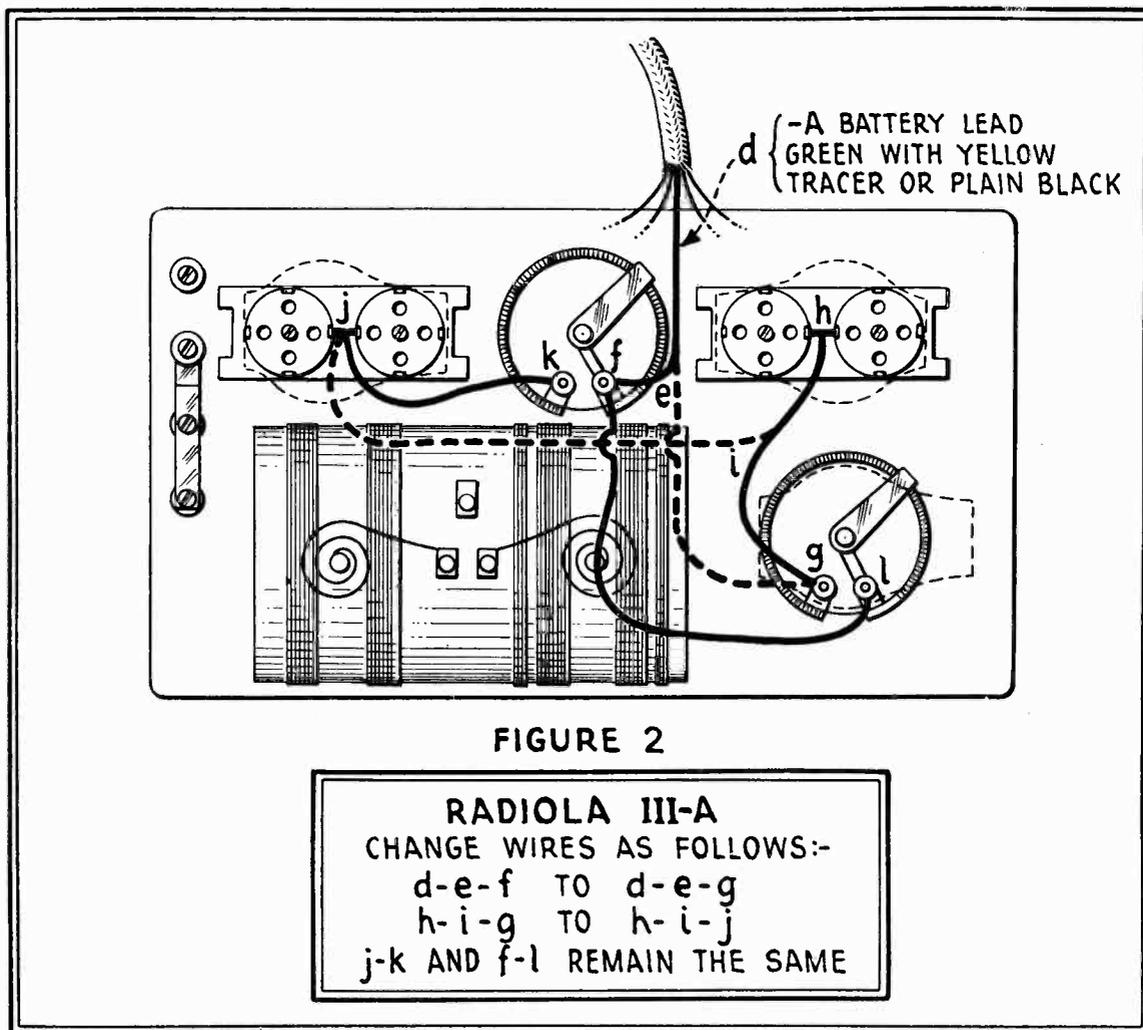
To change wiring of Radiola III-A refer to Figure 2 and proceed as follows:
