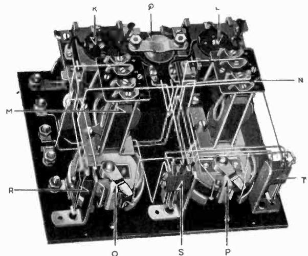
Fig. 2—Radiola AC Audio Amplifier, showing arrangement of parts
