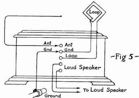
will usually serve the purpose. In making the ground connection, the pipe should be scraped clean and the ground wire firmly connected.
