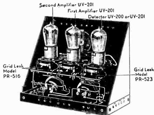
some point the tube will start to oscillate. This condition is denoted by disappearance of the signal and the appearance of a loud mushy sound in the receivers. Turn the "INTENSITY" knob back slightly, until the signals are again loud, and the oscillation of the tube has ceased.
