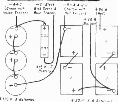
Diagram of Battery Connections for Portable Unit
