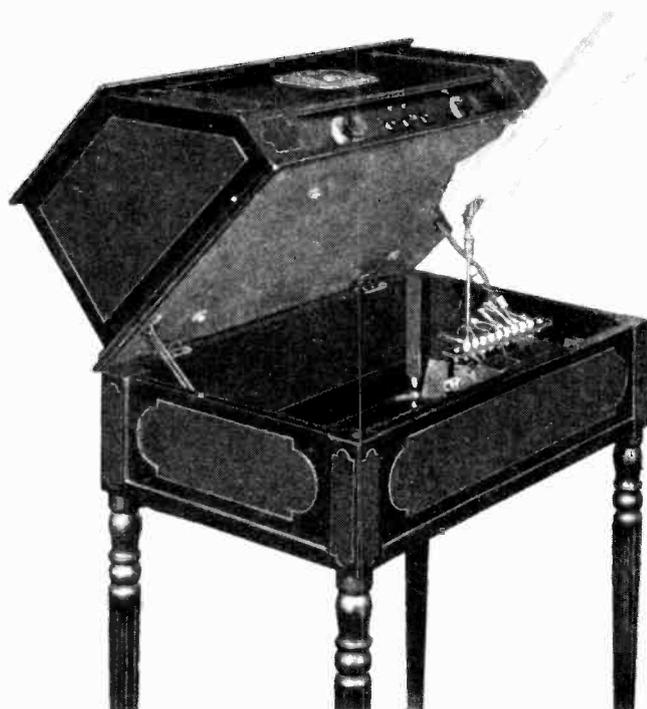
*Figure 5—Installing condenser bank of A.C. Package UP-972*
