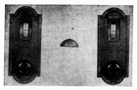
Figure 14—Detailed view of the pilot light socket and canopy. adjust the potentiometer located at the extreme left (facing the front of the Radiola) for position of minimum hum.
