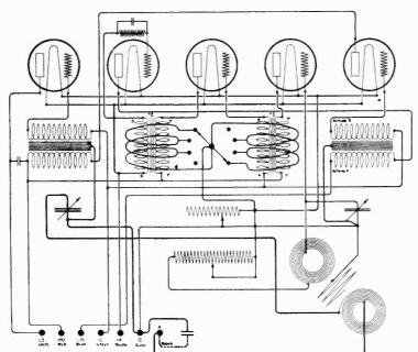
Fig. 6-Schematic Wiring Diagram of Radiola IX
