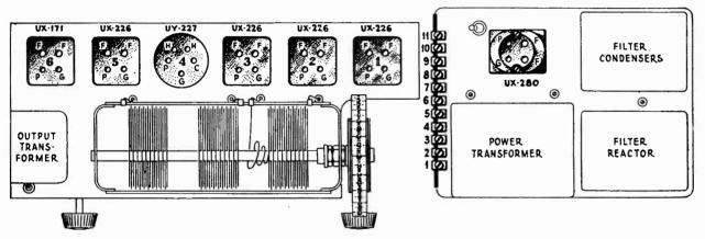
Figure 5—Radiotron socket contacts.
