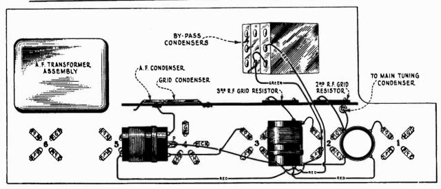
Figure 20-R. F. transformer connections and cotor scheme of wiring.
