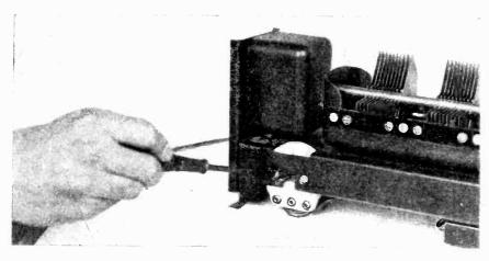
Figure 7—Releasing mounting screws holding volume control.
