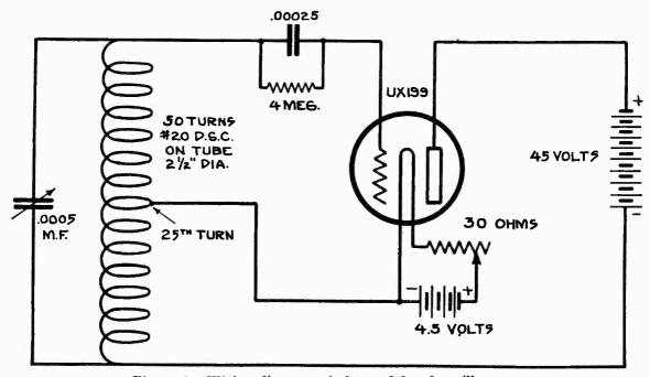
Figure 4-Wiring diagram of the modulated oscillator
