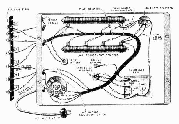
Figure 9-Wiring diagram of Radiola 51 D.C. socket power unit.
