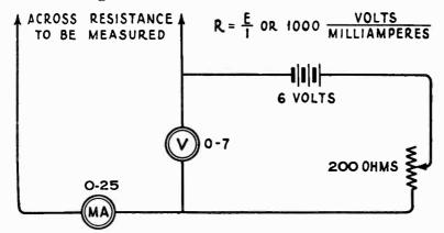
Figure 12-Schematic circuit for resistance measurement.
