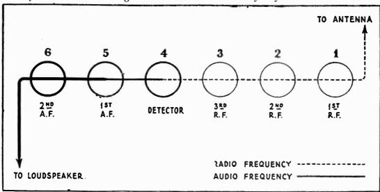
Figure 2-Radiotron sequence in RCA Radiola 16
