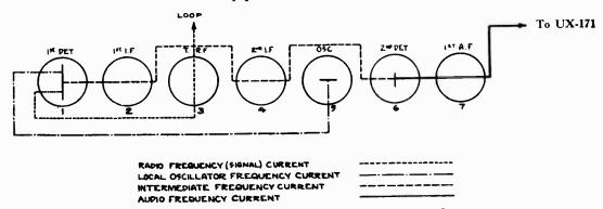
Figure 3—Radiola 30A Radiotron sequence and path of the different currents
