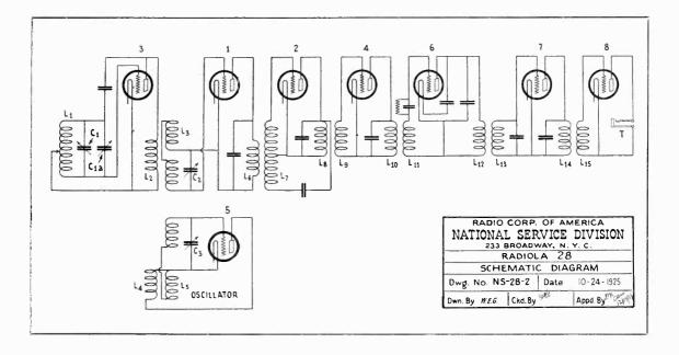
This circuit diagram is not intended for use in checking continuity tests. Use the continuity wiring diagram illustrated in Figure 7, page 12, for such tests.
