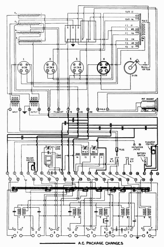
Figure 4—Radiola 28 A.C. operated continuity circuit diagram
