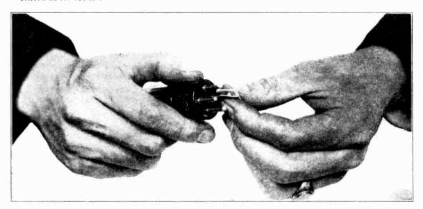
Figure 3—Raditron prongs may be cleaned with fine sandpaper
