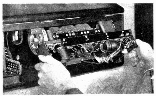
Figure 19—Removing the receiver assembly from the cabinet.
