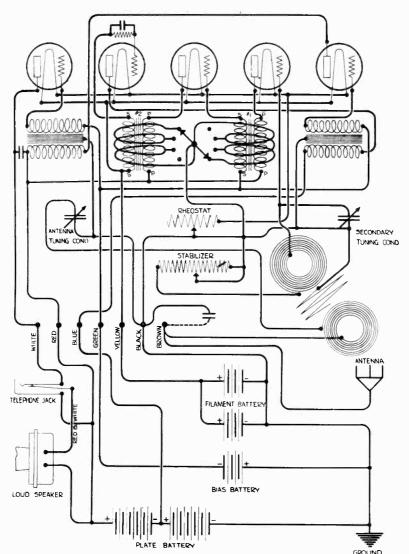
Fig. 4—Schematic Wiring Diagram Radiola VII-B
