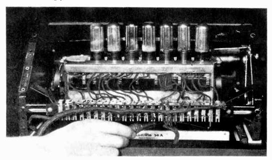
Figure 7-Adjusting neutralizing condenser
