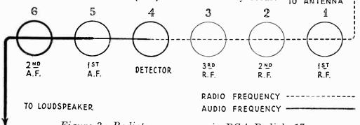
Figure 3—Radiotron sequence in RCA Radiola 17
