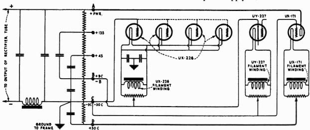
Figure 18—Schematic circuit for securing grid biasing voltages.
