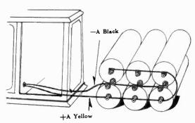
Fig. 3-Showing Method of Connecting A Batteries
