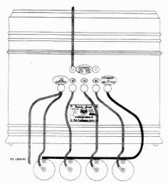
Diagrammatic Connection of Dry Cells
