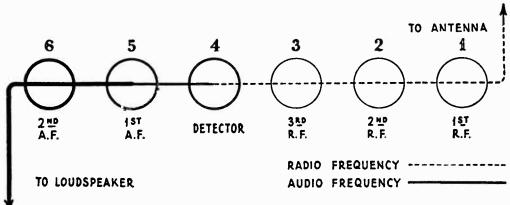
Figure 4—Radiotron sequence in RCA Radiola 18.
