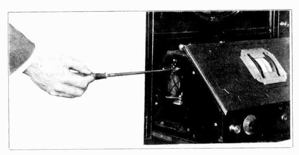
Figure 5-Adjusting the compensating condenser with a non-metallic screw-driver
