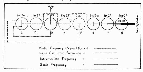
Figure 1—Radiola 28 Radiotron sequence
