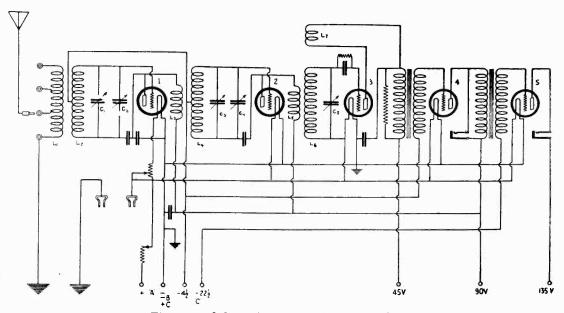
Figure 1 -- Schematic circuit of RCA Radiola 20
