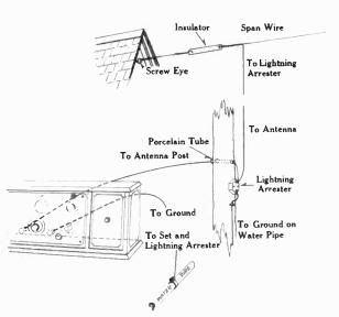
Fig. 2-Showing Connections to Antenna, Ground and Lightning Arrester
