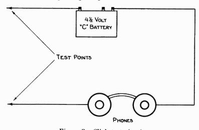
Figure 3—Click test circuit
