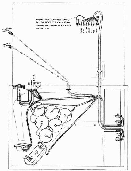
Fig. 3—Cable Connections of Radiola VII-B LOUD Speaker, Jack and Batteries
