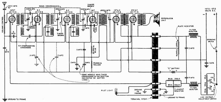
Figure 5—Schematic circuit diagram of Radiola 51 D.C.
