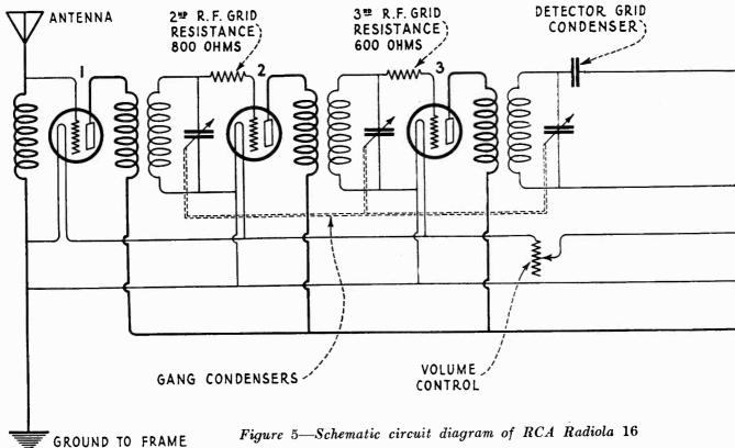
Figure 5-Schematic circuit diagram of RCA Radiola 16
