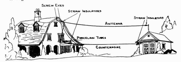
Figure 3—Typical Outdoor Antenna Installation (Showing use of counterpoise where good ground is not available)
