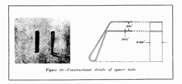
armature correctly it will be first necessary to make a set of spacer tools (Figure 10). These are made of ½" stock phosphor bronze .010" thick and bent to give two surfaces .091" apart. Two of these tools are necessary. After the two screws are loosened at each end of the armature these tools are inserted at each end between the armature and pole pieces (Figure 11). The screws are then tightened with the spacer tools in place. This completes the adjustment.
