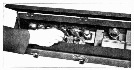
Figure 6—Adjusting the compensating condenser.
