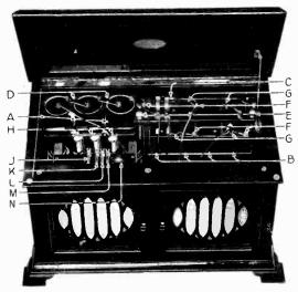
Fig. 1 Interior View Showing Battery Connections
