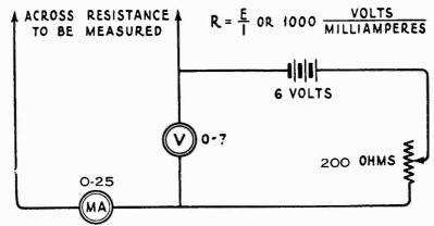
Figure 6-Schematic circuit for resistance measurement
