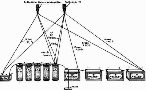
Fig. 1-Showing Connections for Batteries
