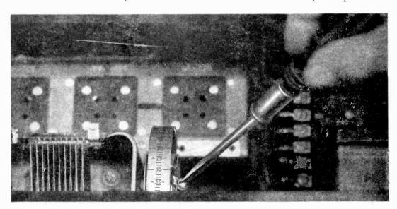
Figure 9—Turning cable adjusting screw to take up slack in tuning drum cable.
