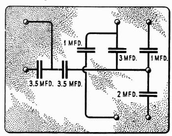
Figure 17—Internal connections of filter condensers.
