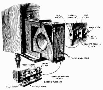
Figure 8.4—Method of insulating reproducer unit from cabinet to prevent microphonic action
