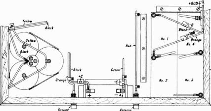
Fig. 2-Diagram of Battery Connections
