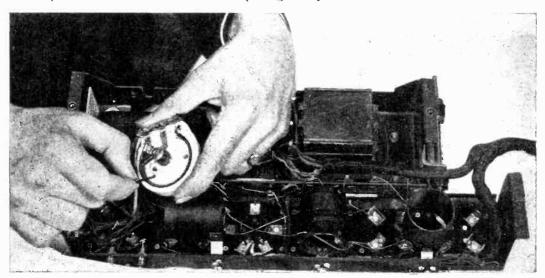
Figure 8—Adjusting the contact arm to secure improved contact with resistor strip.
