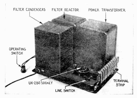
Figure 2—Socket Power Unit showing various parts.
