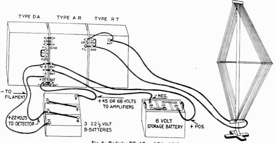
Fig. 6-Radiolas RT, AR and DA with Loop
