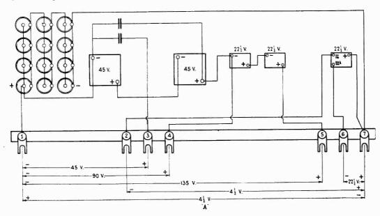
Figure 6—Correct voltage readings across battery terminal strip
