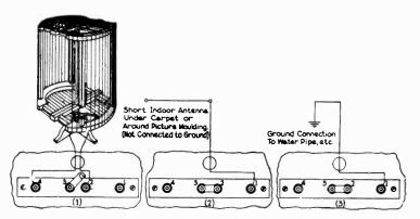
Fig. 5. Connection of Exterior Loop, Indoor Antenna, etc.
