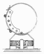
Fig. 3-View Showing Top of Antenna Coil
