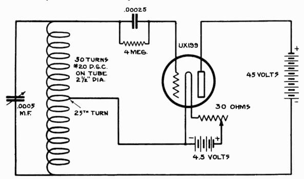
Figure 4-Wiring diagram of the modulated oscillator
