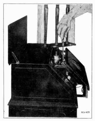
Figure 5—Adjusting the loop compensating condenser
