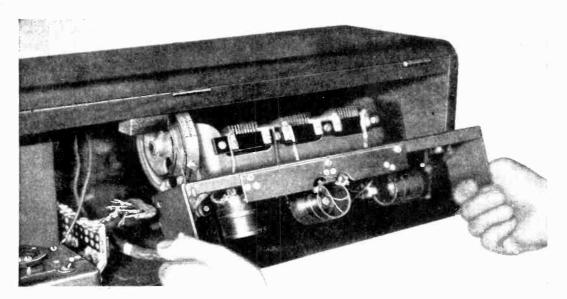
Figure 12—Removing receiver chassis assembly from cabinet.
