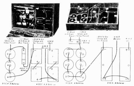
Diagram of Battery Connections for Portable Unit -Diagra
