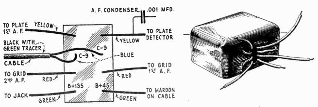
Figure 10-Audio frequency transformers and color scheme of connections
