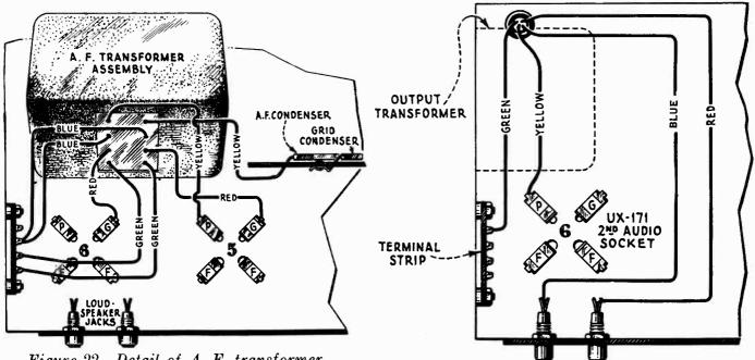
Figure 22—Detail of A. F. transformer connections and color scheme of wiring.
