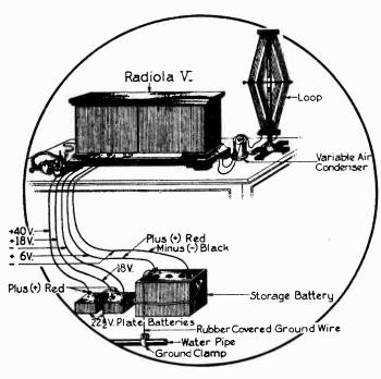
to the negative (-) of the 40-volt plate battery, omitting the connections from the "-40 V." terminal of the receiver to the plate battery.
