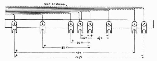
Figure 2-Radiola 25 Battery Terminal Strip
