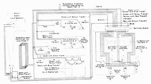
Fig. 5. Connection Diagram of Radiola Super-VIII
