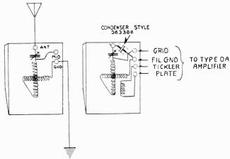
Fig. 3-Diagram of Connections for Radiolas RT andRA
