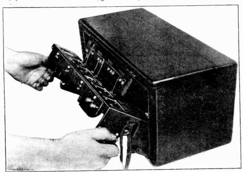
Figure 8-Removing chassis assembly from cabinet
