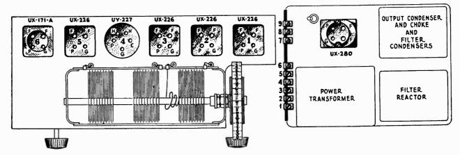
Figure 5—Radiotron socket contacts.
