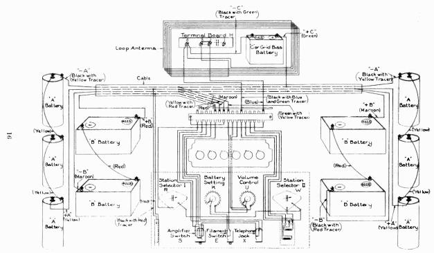
Fig. 6.—Connection Diagram of Radiola Super-Heterodyne
