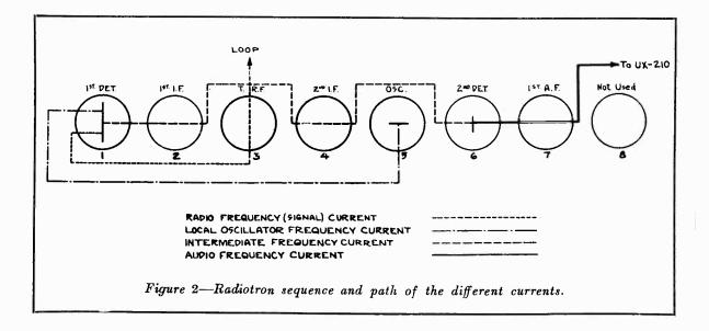
From Radiotron No. 4 the signal is fed into No. 6, which is the second detector. The audio frequency current is now fed through Radiotron No. 7 and Radiotron UX-210 in the R. P. A. unit. Figure 2 illustrates the Radiotron sequence and the path of the different currents through them.
