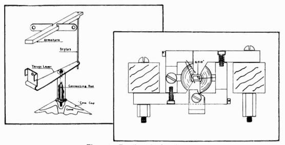
Figure 9-Details of loudspeaker unit
