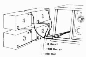
Fig. 4-Showing Method of Connecting B Batteries
