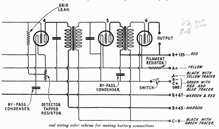
reducing them to 67 volts. Off hand it would seem that a series resistance could be used to drop the voltage, but when we realize the plate voltage varies in practically all of these devices except in the case of the RCA "B" Eliminator (Duo-Rectron) and similar devices a fixed resistor would give a varying voltage depending on the device.
