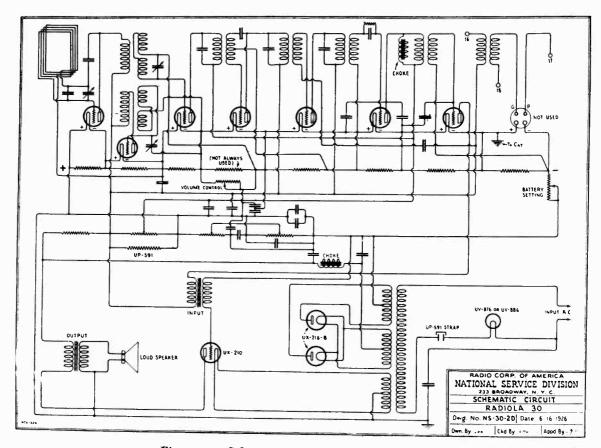
Figure 13:-Schematic circuit diagram of Radiola 30
