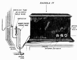
Fig. 2. Installation of Radiola IV
