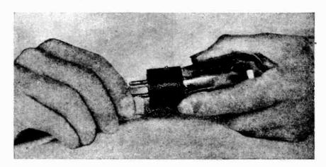
Figure 6-Method used to clean Radiotron prongs.
