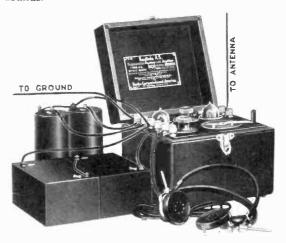
Fig. 2-Radiola RS Connected
