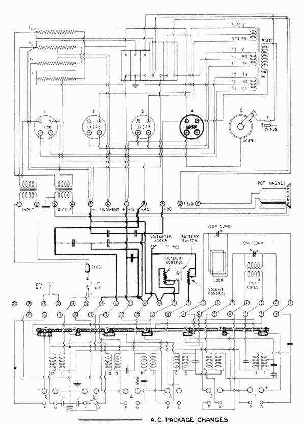
Figure 1—Radiola 25 A.C. operated continuity circuit diagram
