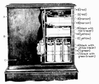
Fig. 1. Rear View, Showing Battery Connections
