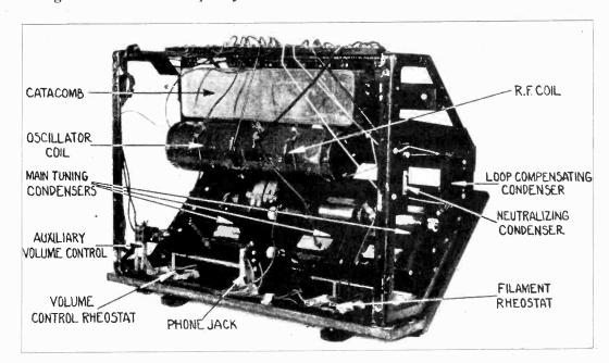
Figure 2—Rear view of panel assembly
