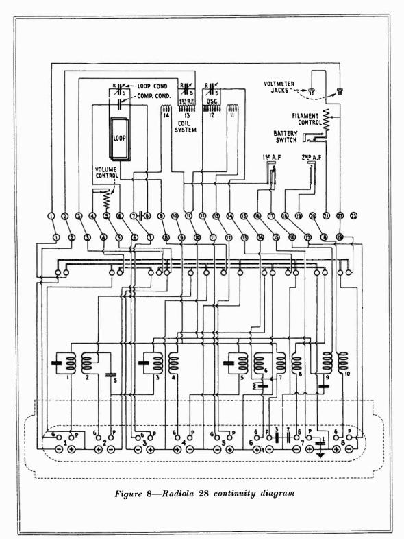
The contacts of the test equipment should be placed across the terminals indicated under the colum marked "Terminal" and the results should be as indicated under the column marked "Correct Effect." If the results are negative the cause of such negative effect will be found in the last column under the heading "Incorrect Effect Caused By." The first colum indicates the circuit under test.
