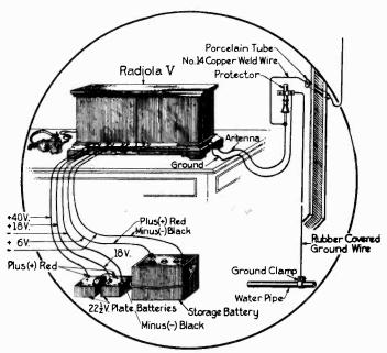
receiver as possible. When using Radiotron UV-200 as a detector, make the battery and other connections as indicated on the diagram. When Radiotron UV-201 is used as a detector, omit the lead from the 18-volt terminal of the battery and connect together the "+18 V." and "+40 V." terminals on the rear of the receiver.
