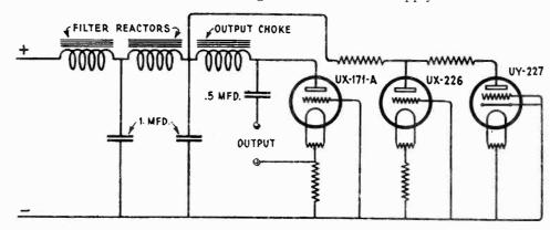
Figure 9—Schematic circuit illustrating method of obtaining grid and plate voltages.
