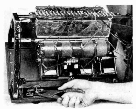
Figure 4-Adjusting contact arm on rheostat
