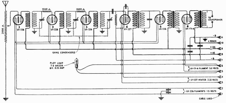
Figure 4-Schematic circuit diagram of receiver assembly.
