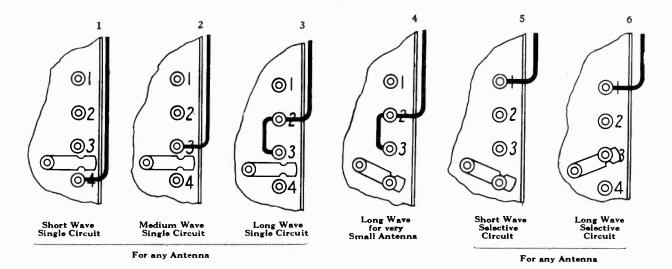
Fig. 3—Showing Antenna Connections to Different Binding Posts
