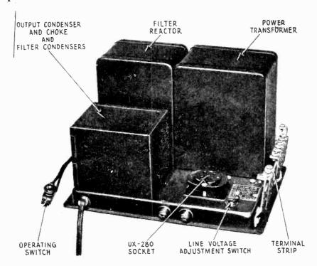
Figure 2—Socket power unit showing various parts.
