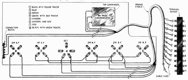
Figure 25—Color scheme of power cable connections.
