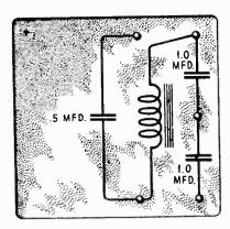
Figure 8—Internal connections of condensers.
