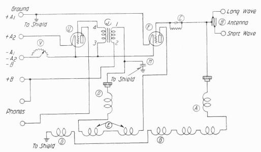
Fig. 6-Diagram of Connections Radiola RS
