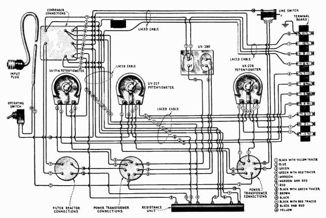
Figure 16—Continuity wiring diagram of socket power unit and color scheme of wiring.
