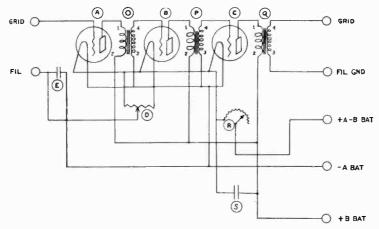
Fig. 4-Diagram of Connections of Radiola AR
