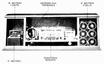
Fig. 5 Internal View of Radiola Regenoflex
