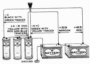
Fig. 2-Battery Connections
