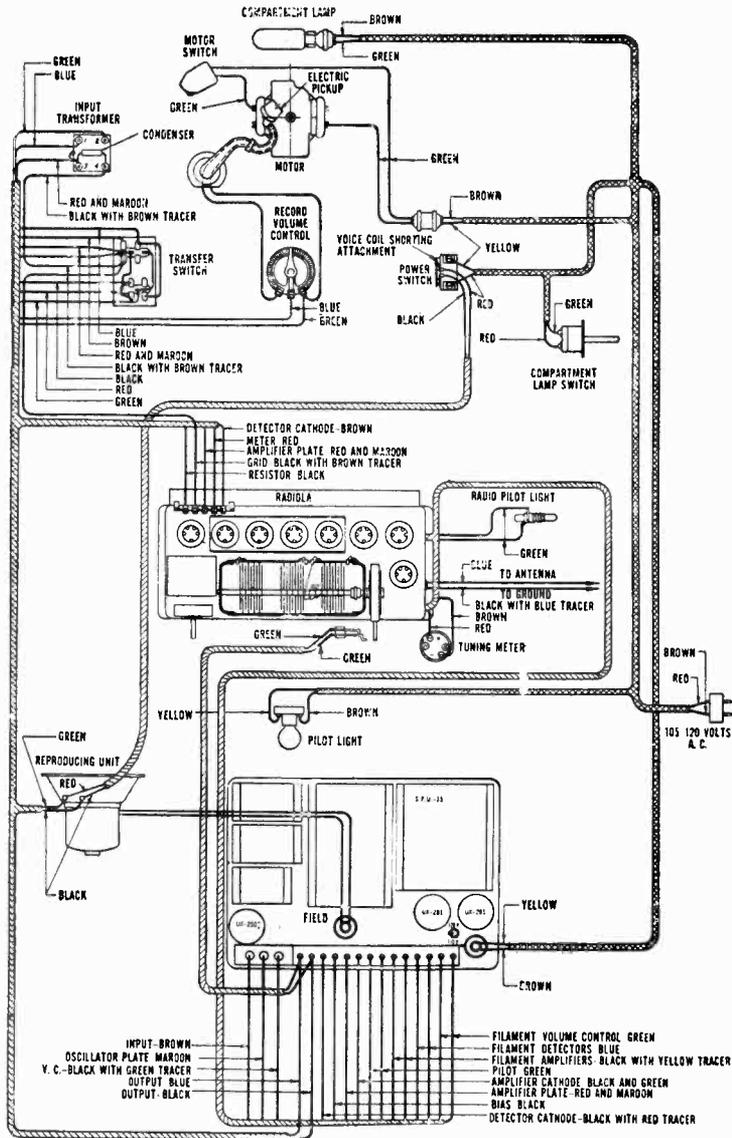
Cable Wiring Diagram Electrola Radiola No. 9-18
