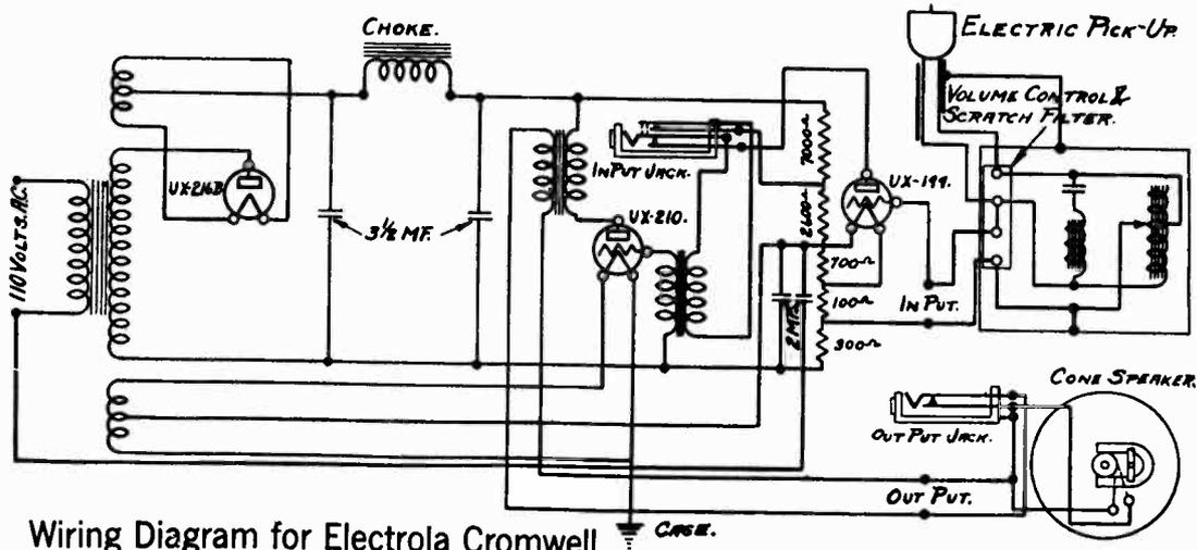
Wiring Diagram for Electrola Cromwell
