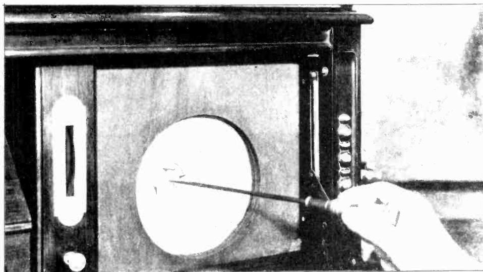
*Figure 11—Method of adjusting the cone. Note the three pieces of cardboard used in centering the cone*
