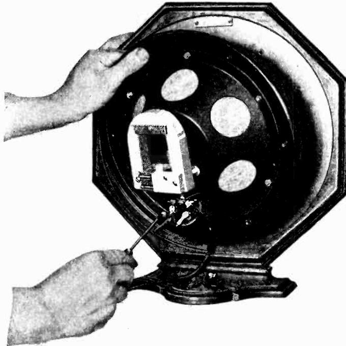
*Figure 11—Removing reproducer assembly from baffle*
