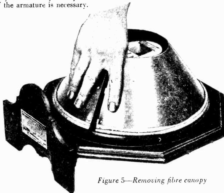
*Figure 5—Removing fibre canopy*
