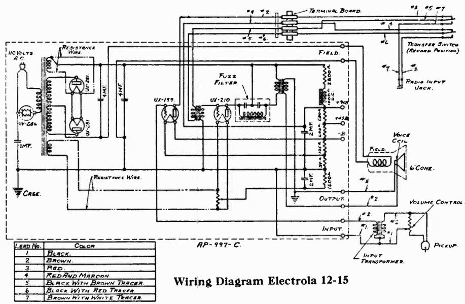
Wiring Diagram Electrola 12-15
