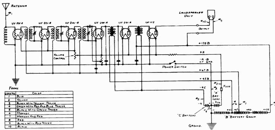
Wiring Diagram for Victor Radiola 16
