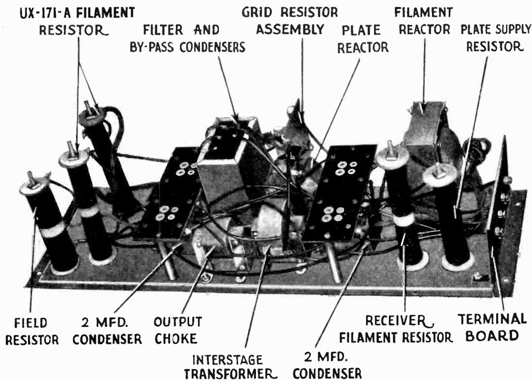
Figure 4—Socket power unit, showing parts
