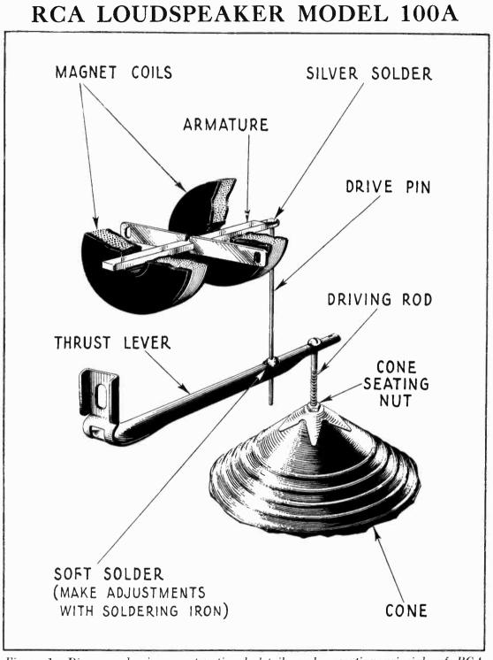
Figure 1-Diagram showing constructional details and operating principle of RCA Loudspeaker 100A
