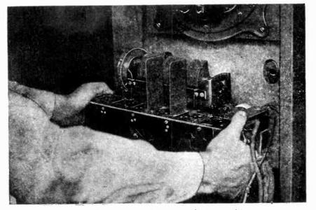
Figure 20—Removing receiver assembly from cabinet
