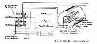
8-60 Input Transformer Wiring
