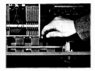
Fig. 4—Method of Adjusting Compensating Condenser
