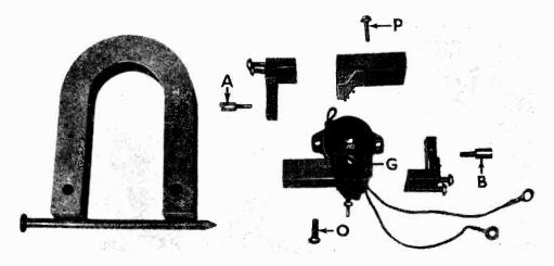
Figure 9-Motor mechanism partly exploded
