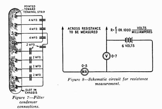
These resistances should be close to their rated values in order to supply correct plate and grid voltages to Radiotron UX-250 for best operation.
