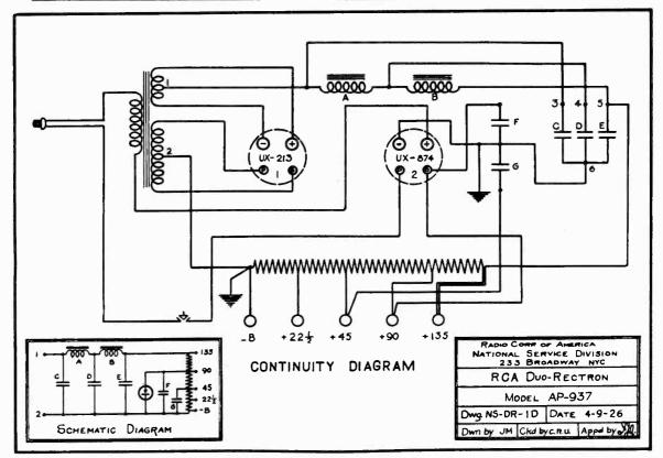
Figure 3—Continuity wiring diagram of RCA "B" Battery Eliminator. 7
