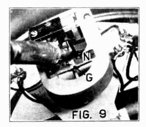
Soldering the stylus to the thrust lever
