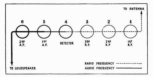
Figure 3—Radiotron sequence
