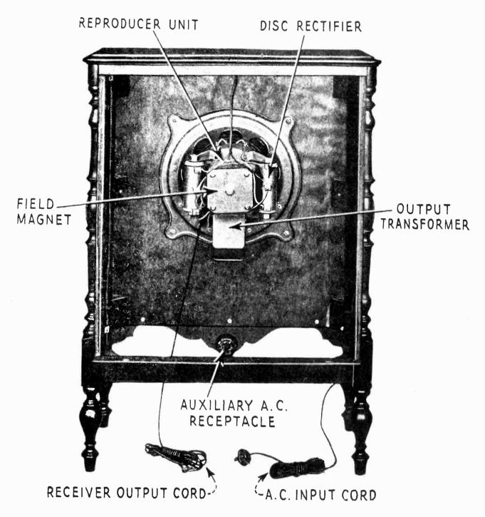
Figure 1-Rear interior view of Loudspeaker 106
