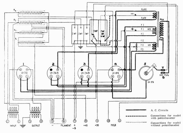
Figure 7-Continuity circuit of R.P.A. Unit
