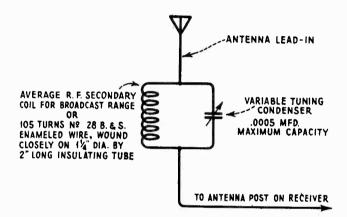
Figure 8-Schematic diagram of wave trap
