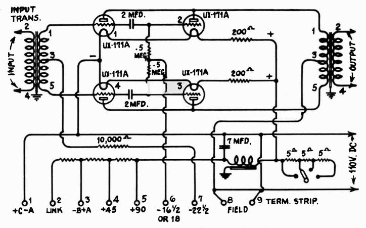
Figure 4 -- RCA Loudspeaker 104 D.C. socket power unit schematic circuit with terminal connections and "A", "B" and "C" Voltages.
