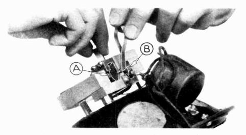
Figure 5—Armature bracket adjusting screws A and B
