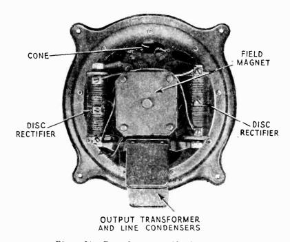
Figure 21—Reproducer assembly showing parts
