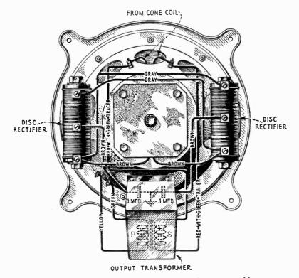
Figure 10-Wiring diagram of reproducer assembly
