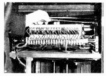
Figure 6-Adjusting the loop compensating condenser
