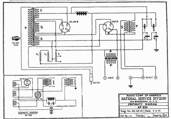
Figure 4 Continuity diagram RCA Uni-Rectron
