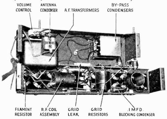
Figure 3-Sub-chassis view of receiver, showing parts
