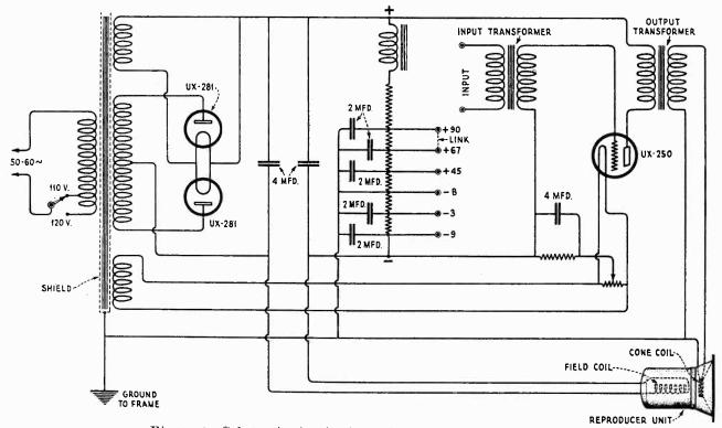
Figure 4-Schematic circuit diagram of RCA Loudspeaker 105.
