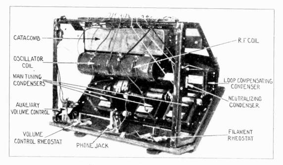
Figure 3-Rear view of panel assembly
