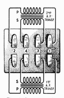
Figure 9—Internal connections of audio transformers
