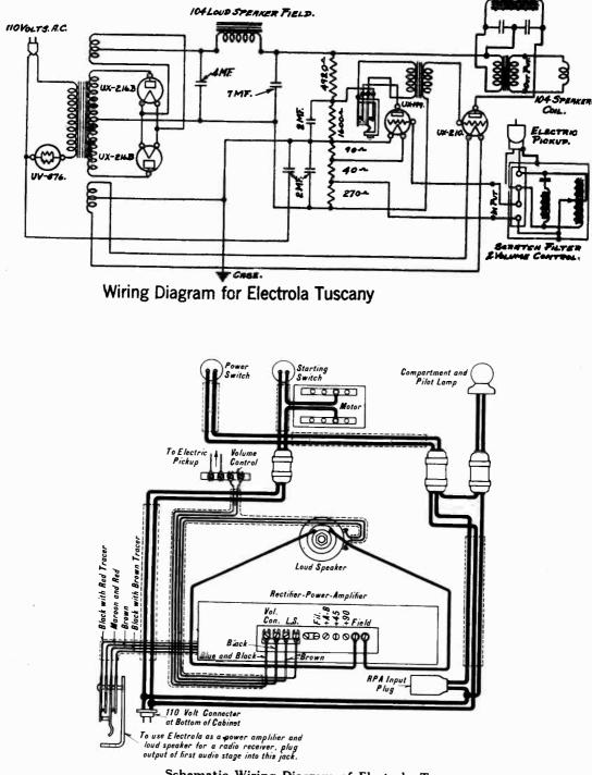
Schematic Wiring Diagram of Electrola Tuscany
