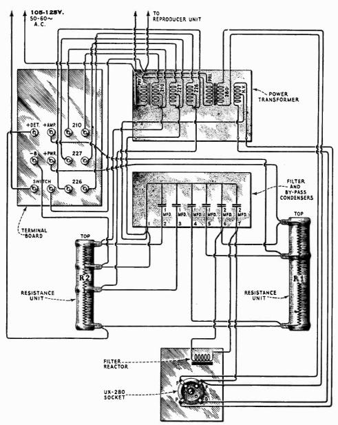
Figure 17—Wiring diagram of Sterling S. P. U.
