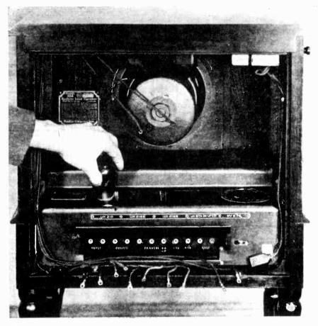
Figure 6—Removal of R.P.A. connections, Radiotrons and Rectrons preparatory running continuity tests
