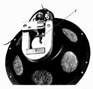
Figure 8—Drive-pin thrust-lever soldered connection (F)
