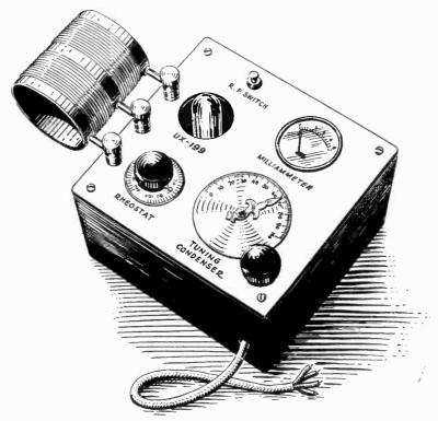
Figure 5-Complete model of R.F. and A.F. oscillator
