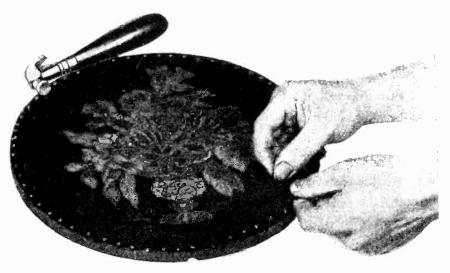
Figure 14—Tacking the grille tapestry in place on the baffle board
