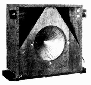
Figure 11-Reproducer unit in housing
