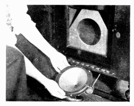
Figure 23—Removing the reproducer from the cabinet
