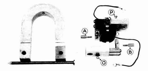
Figure 10-Motor mechanism partly exploded
