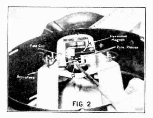
Method of adjusting armature clearance
