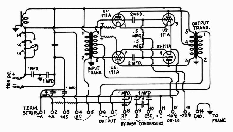
Figure 2 -- Radiola 30A D.C. Socket Power Unit achematic circuit with terminal connections, plate, grid and filament voltages.
