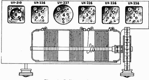
Figure 4-Radiotron socket contacts
