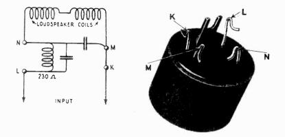
Figure 10—Schematic circuit of Loudspeaker 103 coils and filter and photo of filter unit
