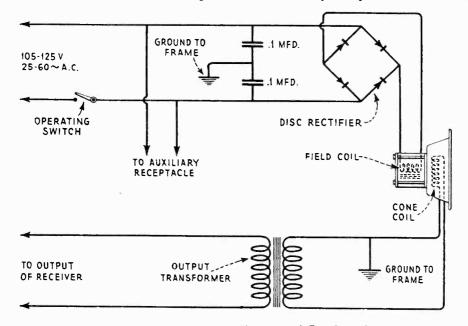
Figure 2-Schematic wiring diagram of Loudspeaker 106
