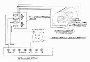
9-40 Input Transformer Wiring
