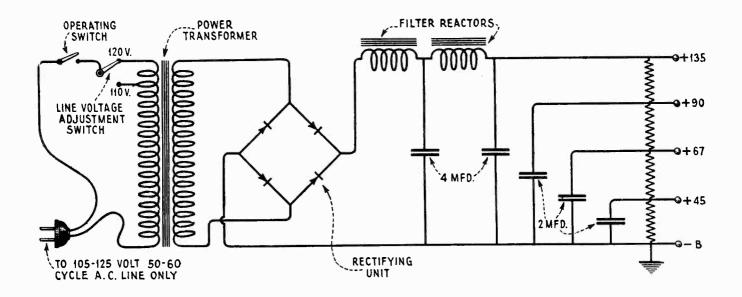
Figure 1-Schematic circuit diagram of RCA B-Eliminator
