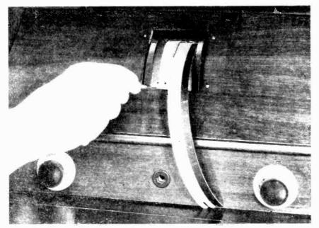
Figure 15-The correct method of replacing dial scales
