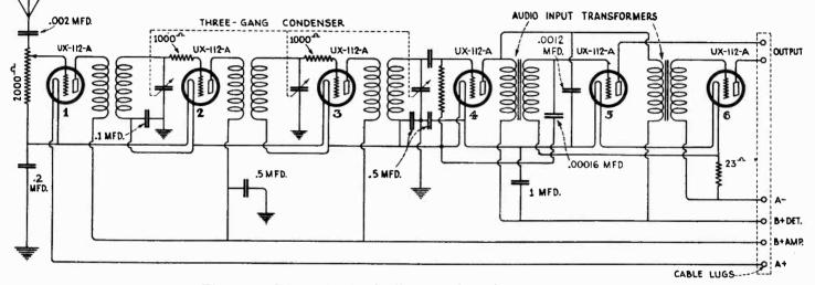
Figure 5-Schematic circuit diagram of receiver
