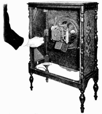
Figure 5-Removing baffle plate
