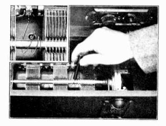
Fig. 7-Method of Adjusting Compensating Condenser
