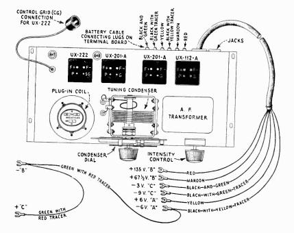
Figure 10-Socket layout and battery cable connections
