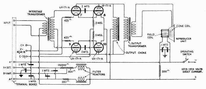
Figure 5A-Schematic circuit diagram of socket power unit
