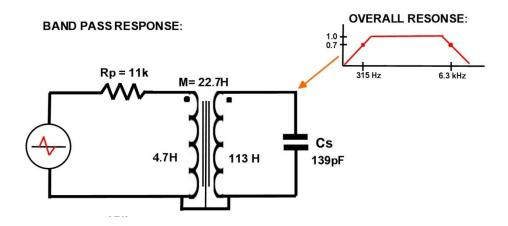
The primary winding can be imagined as coupled into the secondary winding by the mutual inductance M that the two windings share. This coupling alters the resonant properties and damping of the secondary circuit. The influence of the primary winding neutralises the some of the secondary inductance by coupling in an equivalent negative inductance and the degree it does this depends on the resistance in the primary circuit.
