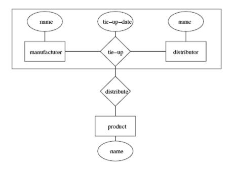
Figure 2.9 E-R diagram Example 2 of aggregation.
