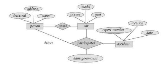
Figure 2.1 E-R diagram for a Car-insurance company.
