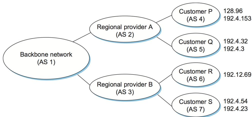
Figure 4.5.: Example of a network running BGP.
