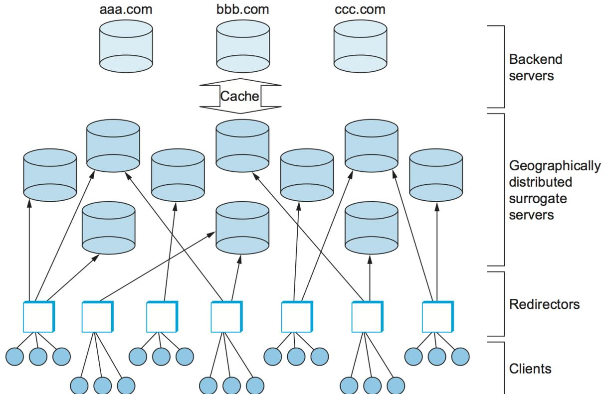
Figure 9.31.: Components in a Content Distribution Network (CDN).
