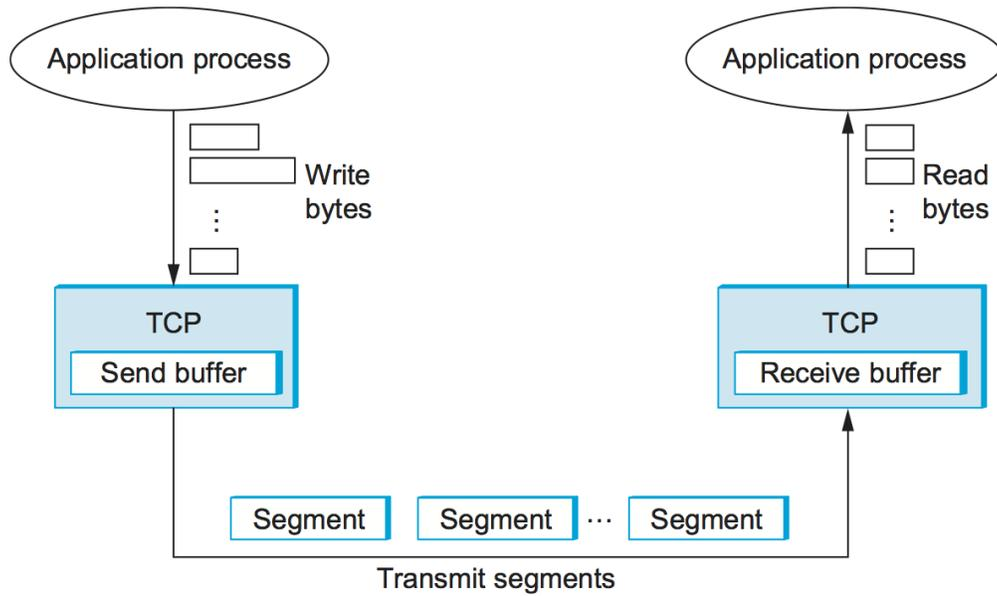
Figure 5.3.: How TCP manages a byte stream.
