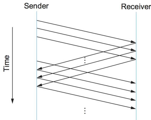
Figure 2.16.: Timeline for the sliding window algorithm.
