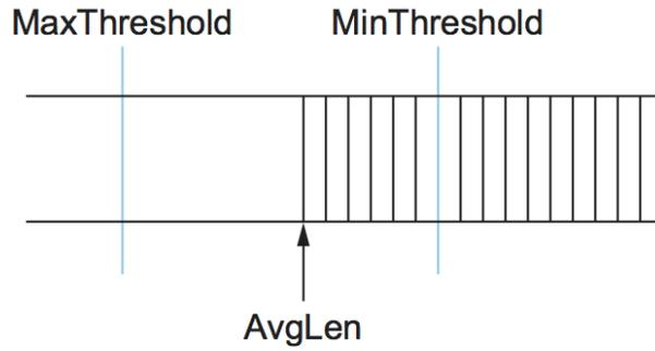
Figure 6.17.: RED thresholds on a FIFO queue.
