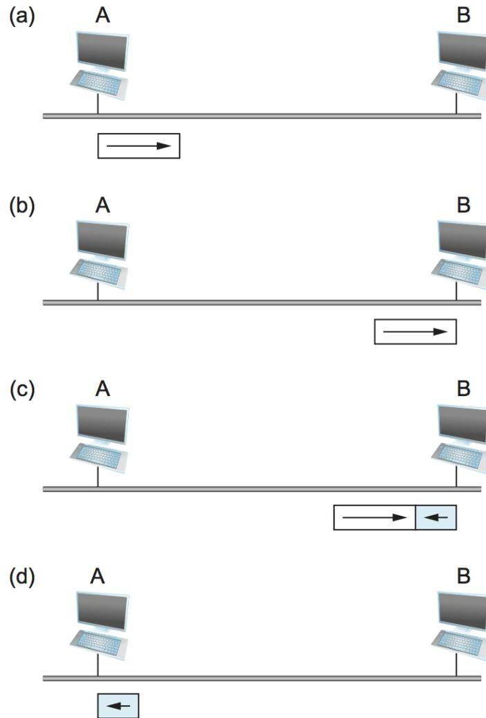
Figure 2.22.: Worst-case scenario: (a) A sends a frame at time  $t$ ; (b) A's frame arrives at B at time  $t+d$ ; (c) B begins transmitting at time  $t+d$  and collides with A's frame; (d) B's runt (32-bit) frame arrives at A at time  $t+2 \times d$ .
