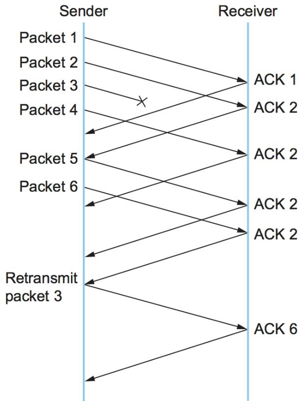
Figure 6.12.: Fast retransmit based on duplicate ACKs.
