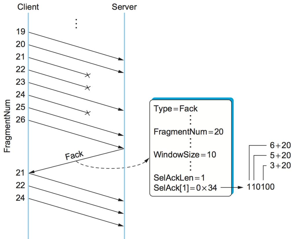
Figure 5.20.: Fragmentation with selective acknowledgments.
