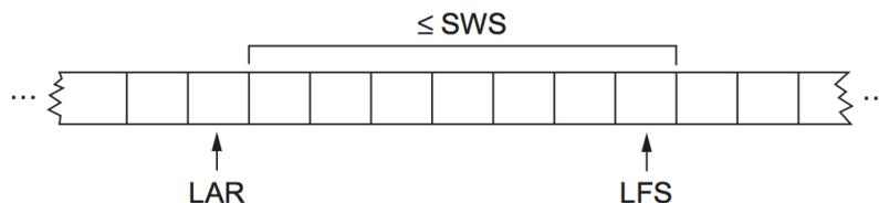
Figure 2.17.: Sliding window on sender.
