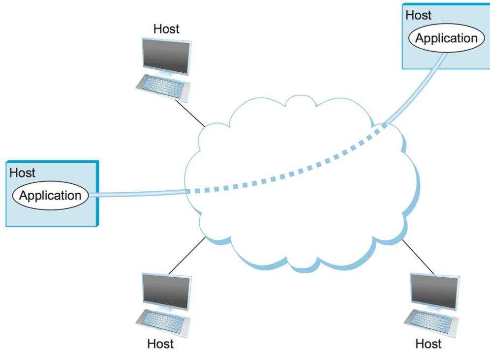
Figure 1.7.: Processes communicating over an abstract channel.
