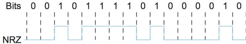
Figure 2.4.: NRZ encoding of a bit stream.
