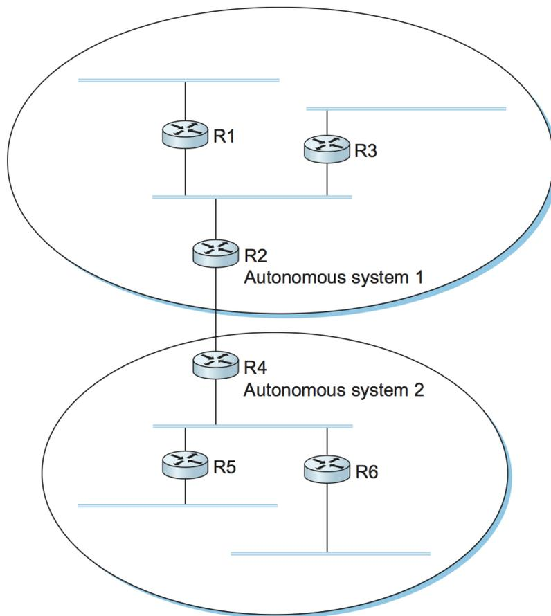
Figure 4.3.: A network with two autonomous systems.
