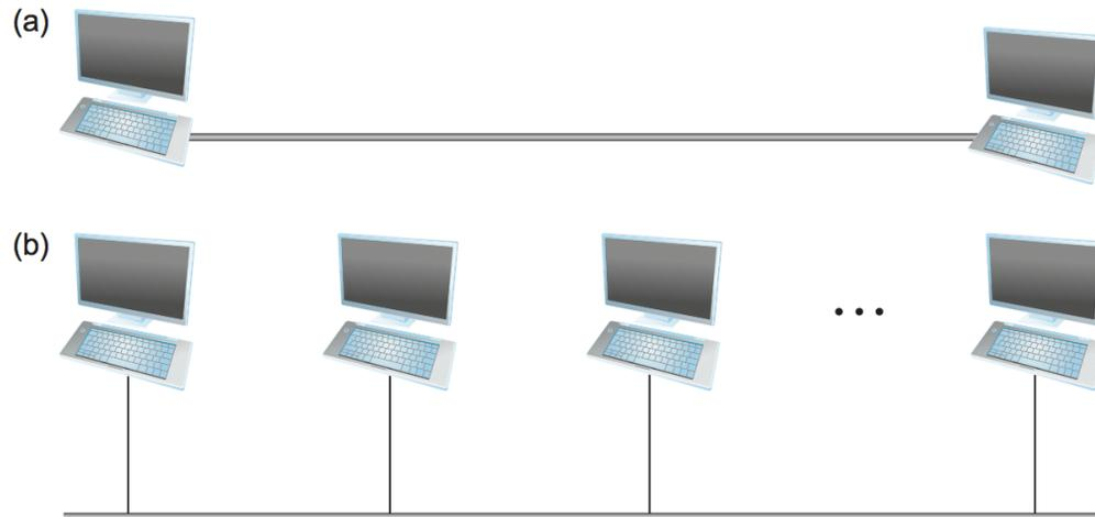
Figure 1.2.: Direct links: (a) point-to-point; (b) multiple-access.
