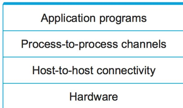
Figure 1.8.: Example of a layered network system.
