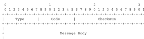
Figure 5.42: ICMP version 6 packet format
