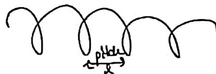
Pitch is dist. moved  $\parallel$  to  $B$  during one revolution
