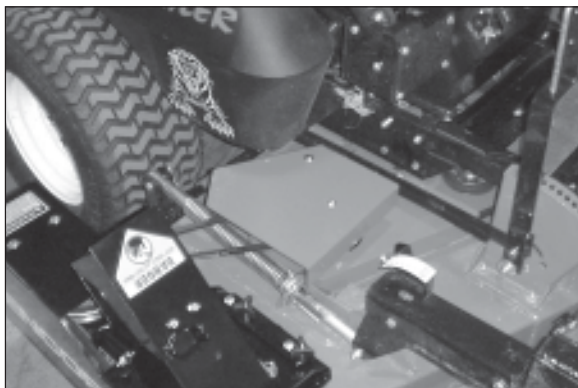
Figure 7 Re-fasten the blower belt shield onto the blower. Also mount the upper RH belt shield to the bracket that is welded to the lower RH belt shield.
