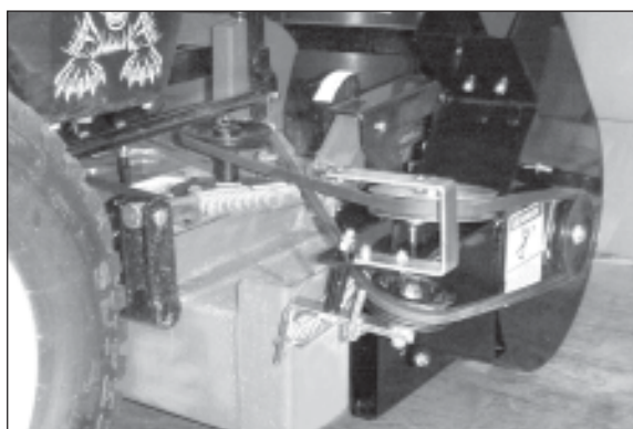
Figure 6 Route the drive belt so that the drive pulley spins the belt in a clockwise direction. Make certain the back side of the belt rides against the tensioner idler and the inside of the V-belt rides against the V-idler. Refer to figure 6 for illustration of belt routing.
