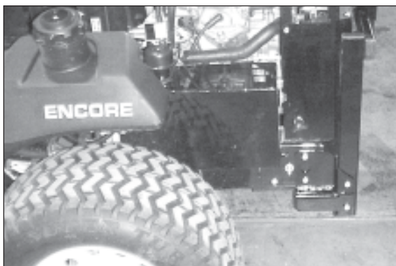
Figure 8b Install the catcher mount weldment found in the blower assembly box to the back end of the frame rails. NOTE: Prowler Midcuts will require the RH & LH catcher adapters to be installed prior to mounting the catcher mount weldment (Figs. 8a & 8b).
