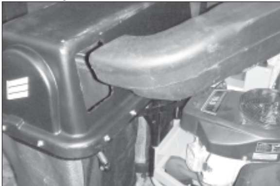
Figure 15 Slide the upper grass tube into the opening of the catcher hood.
