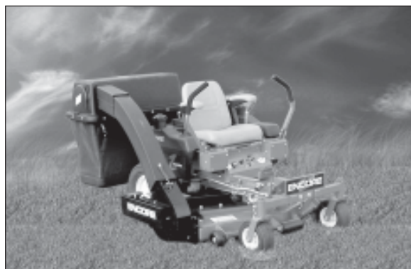
Figure 19 This completes the installation of your new Encore grass catcher system. Note that when engaging the PTO switch; always make certain the unit is running 3/4 to full throttle so as to prevent stalling.
