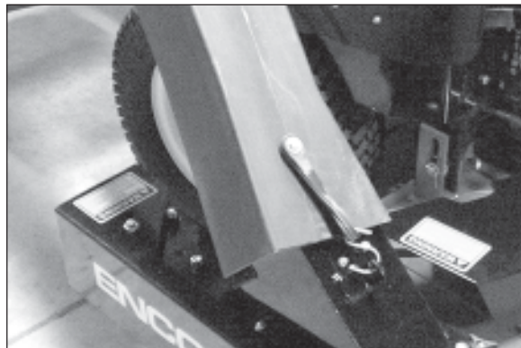
Figure 18 Attach the lower discharge tube to the blower assembly by hooking the tie down strap to the eyelet on the blower.
