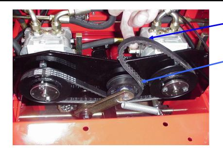
Here is where the pump belt would travel up to and wrap around the engine pulley.
