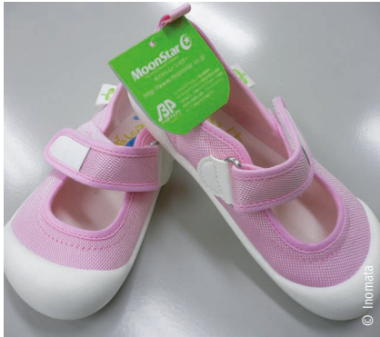
Fig. 4.13: Baby’s shoes made from a PLA/PET blended fabric and soles made from a soft PLA compound [36]
