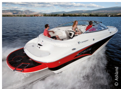
Fig. 4.16: Speedboat made from partially biobased UP resin
