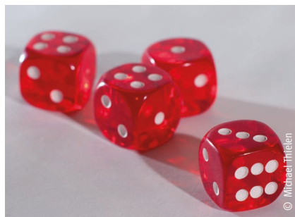
Fig. 4.6: Transparent dice made from cellulose acetate
