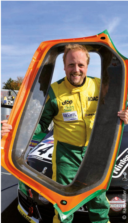
Fig. 6.11: vehicle tailgate made of natural fiber reinforced plastic
