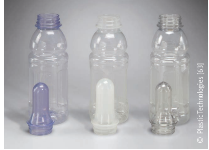
Fig. 5.8: Preforms and bottles (from left to right: PLA, PP, PET)
