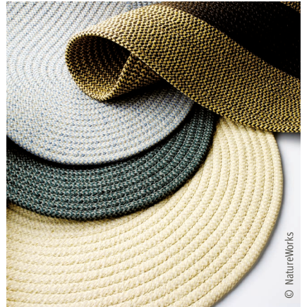
Fig. 6.14: Carpet made from PLA fibers
