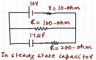
In steady state capacitor will act as a open circuit.
