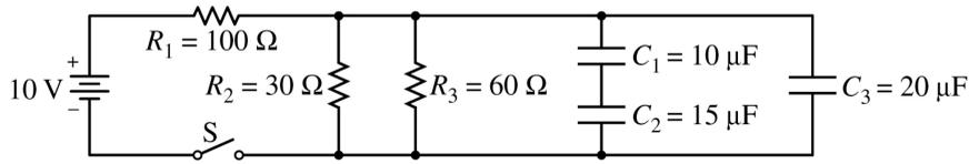
1. The circuit shown above is composed of an ideal 10 V battery, three resistors and three capacitors with the values shown, and an open switch S. The capacitors are initially uncharged. Switch S is now closed.
