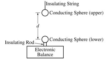
2. Students perform an experiment to study the force between two charged objects using the apparatus shown above, which contains two identical conducting spheres. The upper sphere is attached to an insulating string, which can be used to move the sphere downward. The lower sphere sits on an insulating rod, which is on an electronic balance. The electronic balance is zeroed before the lower sphere and insulating rod are in place.
