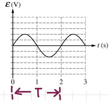
The ring is now mounted on an axle that is perpendicular to the magnetic field. The magnitude of the magnetic field is now held at a constant  $B_0 = 0.50 \text{ T}$ , as shown. The ring rotates about the axle, and the emf  $e$  induced in the ring as a function of time  $t$  is shown on the graph.
