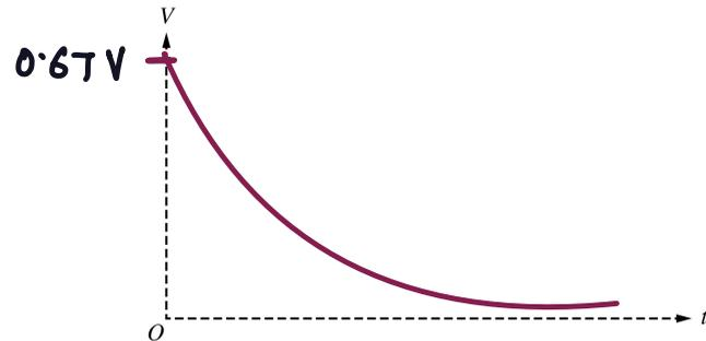
Capacitor  $C_3$  is replaced by two  $10 \mu\text{F}$  capacitors connected in series, switch S is closed, and the circuit reaches equilibrium. Switch S is then opened at time  $t = 0$ .
