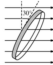
The ring is then rotated so that the plane of the ring is aligned at a  $30^\circ$  angle to the magnetic field, as shown.
