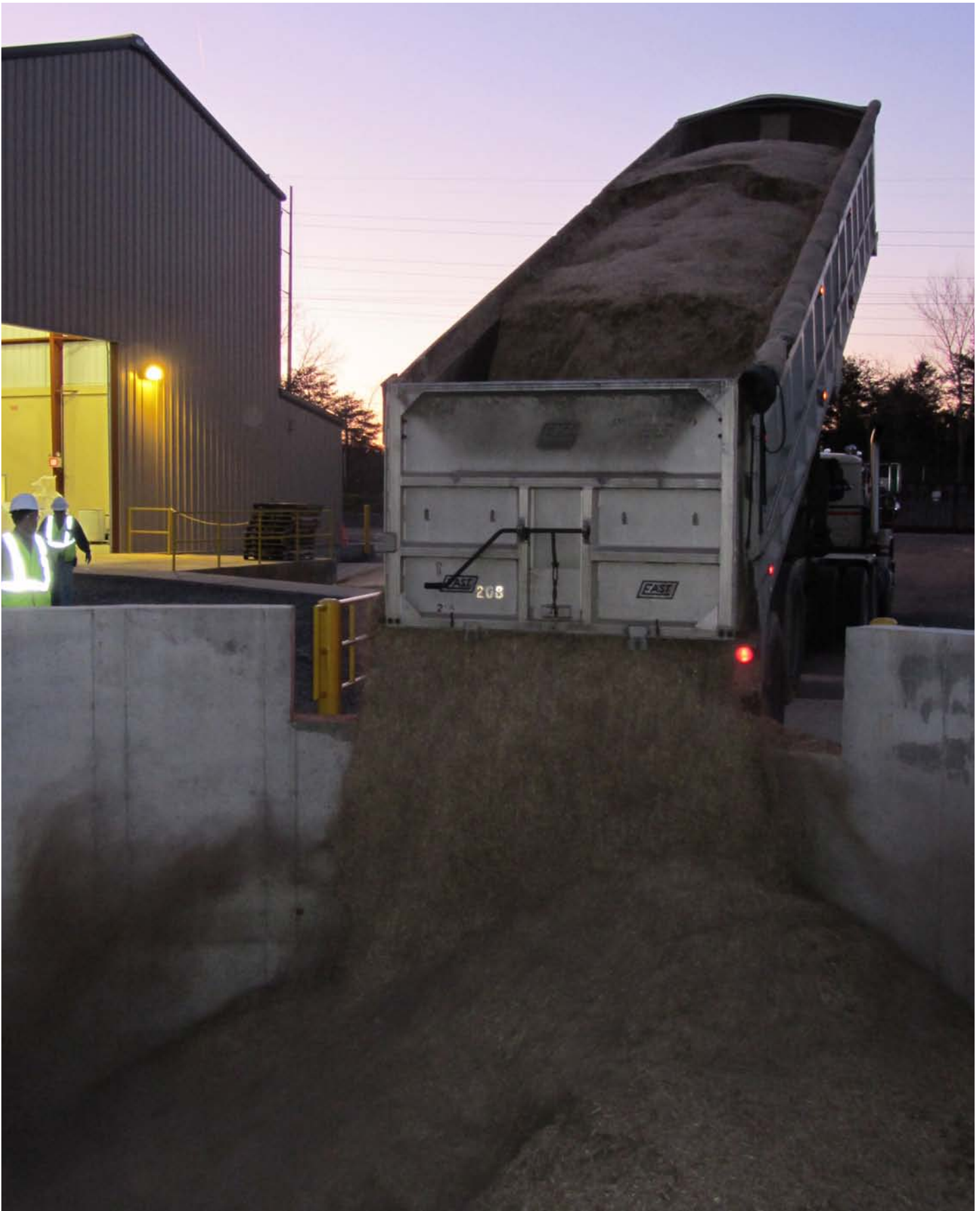
After passing through the forage harvester, low-moisture switchgrass becomes a free-flowing bulk material that can be easily deposited in the receiving pit. Properly timed use of the forage harvester yields better particle size distribution and bulk flow than tub grinding of baled switchgrass. Photo: Al Womac
