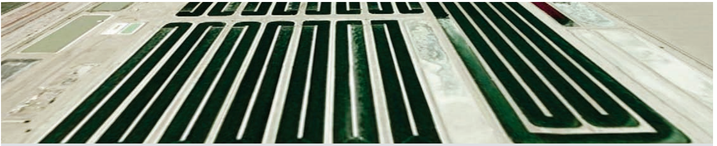
Algae are often grown in outdoor raceway ponds to ensure adequate exposure to sunlight. Research suggests biofuels from microalgae alone could displace 17% of today's transportation fuel imports. Photo: Pacific Northwest National Laboratory (PNNL)
