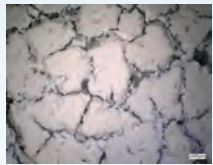
Photograph of the mud-cracking typically observed with ceramic products synthesized at ambient temperature.
