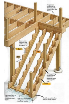
Illustration of customary stair framing
