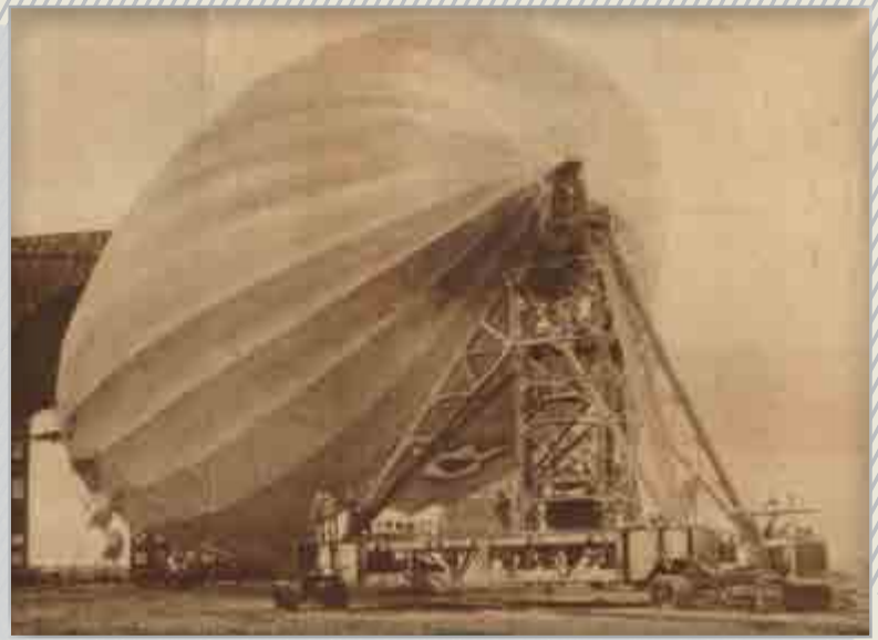
A Cletrac 100 pulling a portable mooring mast at the Lakehurst, New Jersey, Naval Air Station.
