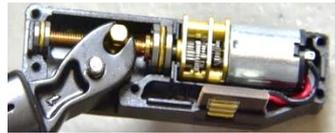
Internal View of Landing Gear Motor
