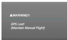
If the Typhoon H loses GPS lock or GPS has been disabled/turned off the Main LED status Indicator on the aircraft will flash purple and the motor LEDs will flash three times per second then off one second and repeat.
