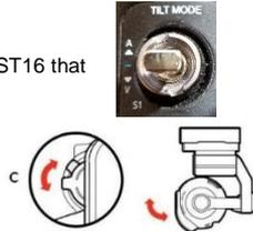
In the **down** position, the Gimbal is in Velocity Mode. Gimbal **tilt rate** (speed) is controllable and the Gimbal is also able to tilt up an additional 15° (degrees) in this switch position.
