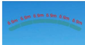
When an **obstacle comes within range**, the [Range] meter (at left) will be displayed on the ST16 with distance to the obstacle. You will also hear a sonar ping. The displayed color will change as you get closer and the pinging will be faster.
