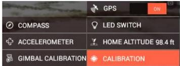
**NOTE:** *The calibration process will take about 2-3 minutes. During the calibration process the gimbal will move around **DO NOT touch or move the aircraft.***
