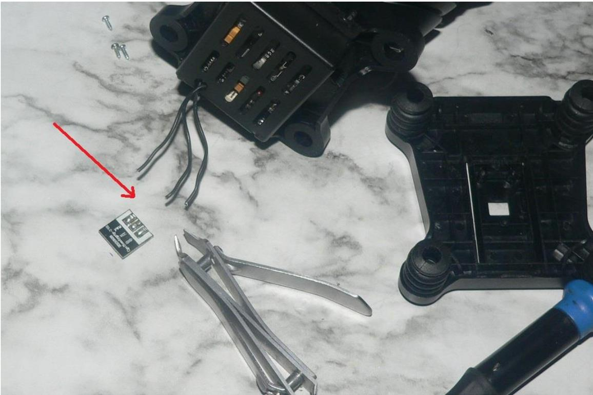
6). Remove both Gimbal Board Enclosure mounting screws:
