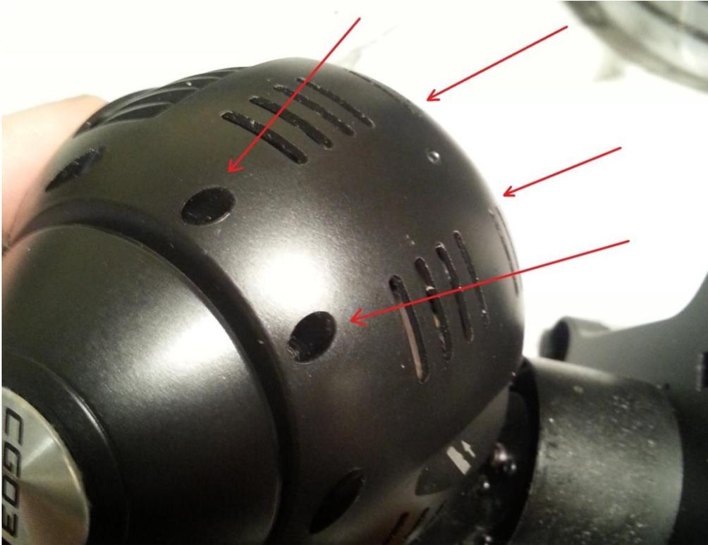
21). Align the front cover, ensuring no wires are trapped between the surfaces or screw mounting holes:
