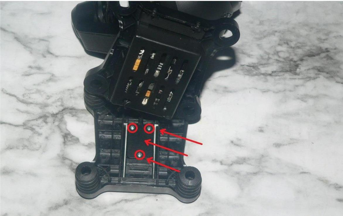
4). Lift Contact Plate out of Upper Camera Mount:
