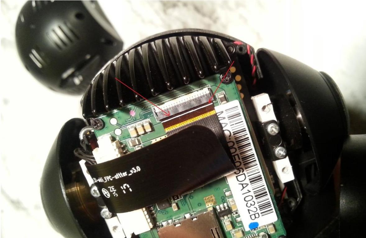
6). Using fingernails or a small tool, lift the back edge of the ribbon lock to release the ribbon:
