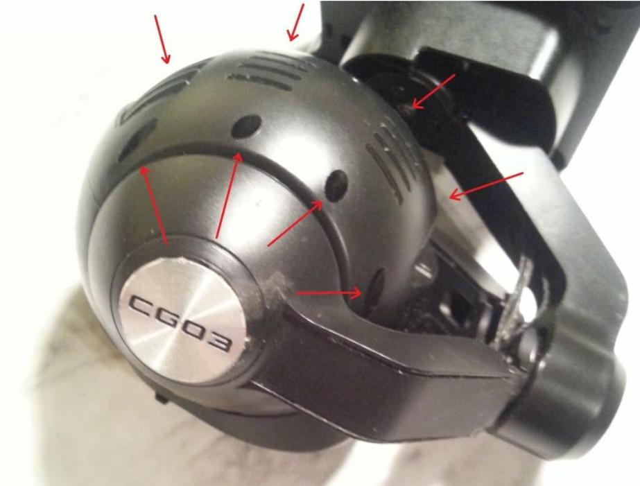
2). Work rear cover slightly forward to clear the USB and SD Card connectors:
