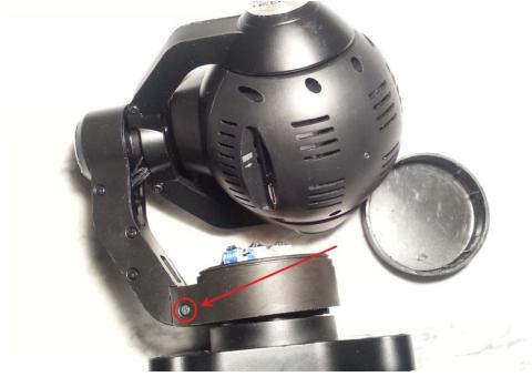
**Note**: Take full advantage of the gap in the enclosure to clear the connectors. Again, rotate camera as needed to maximize available clearance. Do not apply significant pressure. Work with the angles until the enclosure comes free with as little force as possible.
