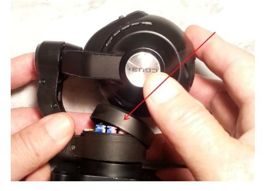
**Note**: Rotate camera as needed to maximize available clearance. Do not apply significant pressure. Work with the angles until the cover comes free with as little force as possible.
