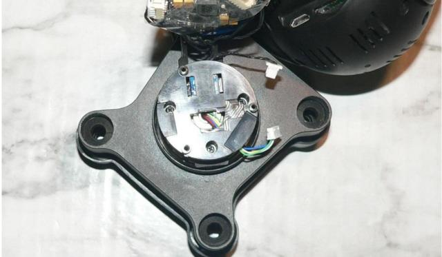
24). Remove temporary strap and lay gimbal board on support:
