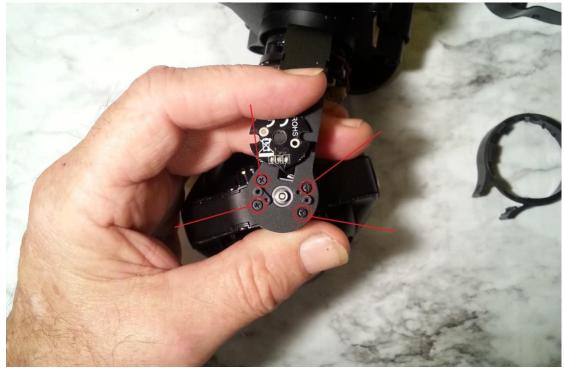
10). Slide the roll motor / camera yoke out of the rear arm:
