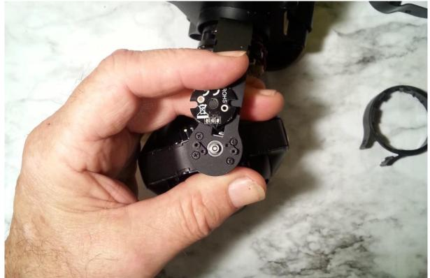
9). Remove the four roll motor screws:
