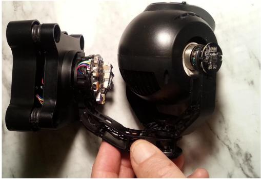
30. Install the Pitch Arm Cover and the two screws at the hub:
