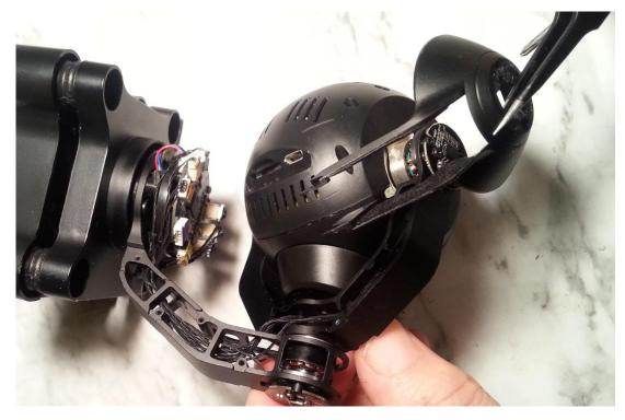
18. Locate the Pitch (tilt) Encoder connector:
