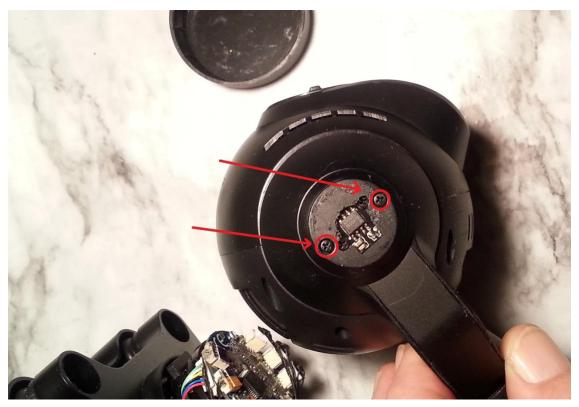
7. Remove the screws from the lower wire cover:
