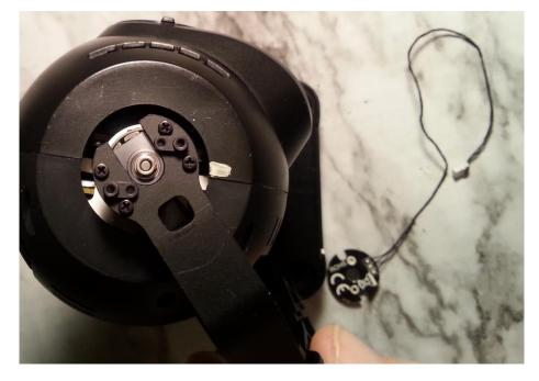
23. Thread the new encoder wire in through the square hole in the Encoder Arm:
