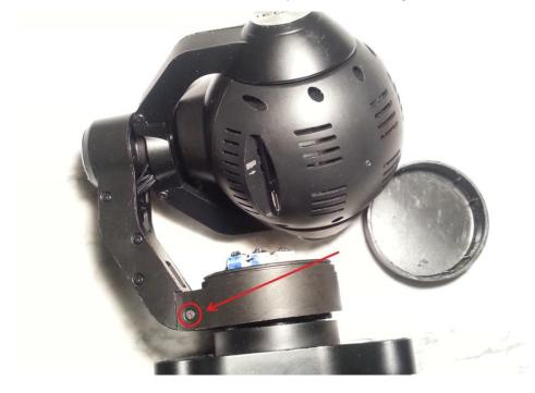
**Note**: Rotate camera as needed to maximize available clearance. Do not apply significant pressure. Work with the angles until the cover is aligned with the Gimbal Board Enclosure:
