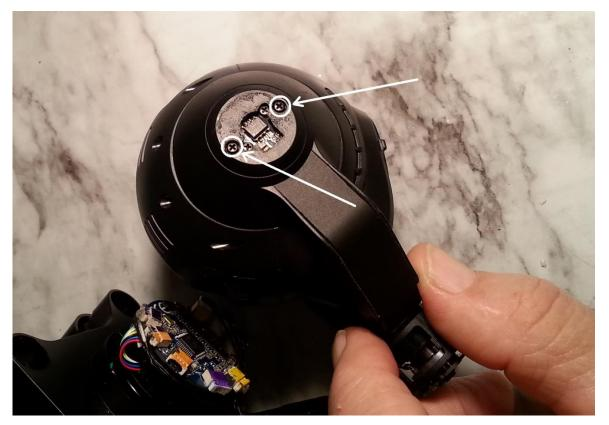
31. Install the Rear Arm Cover and the two screws at the hub:
