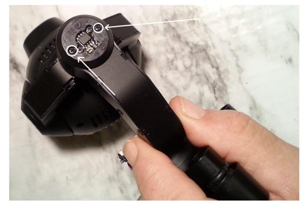
32. Install the screws on both sides of the rear arm cover:
