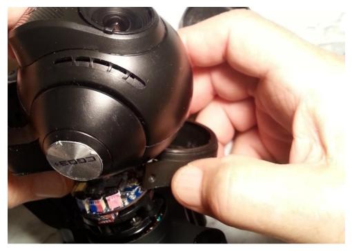
**Note**: Use fingernails or plastic tool to pry the Gimbal Board Enclosure arms over the rear arm tabs.
