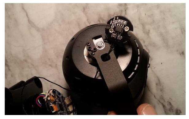
24. Mount the Pitch(tilt) encoder and install the mounting screws:
