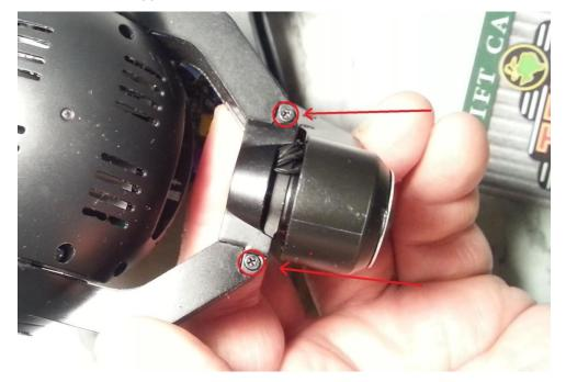
**Note**: Take full advantage of the gap in the enclosure to clear the connectors. Rotate camera as needed to maximize available clearance. Do not apply significant pressure. Work with the angles and move the enclosure into position over the gimbal board.
