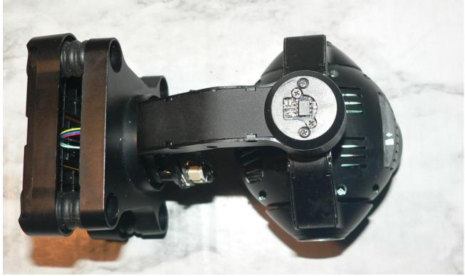
31). Install these three rear arm cover side screws on each side::
