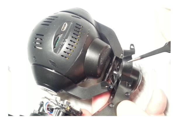
11. Remove these screws from both sides of the rear arm cover:
