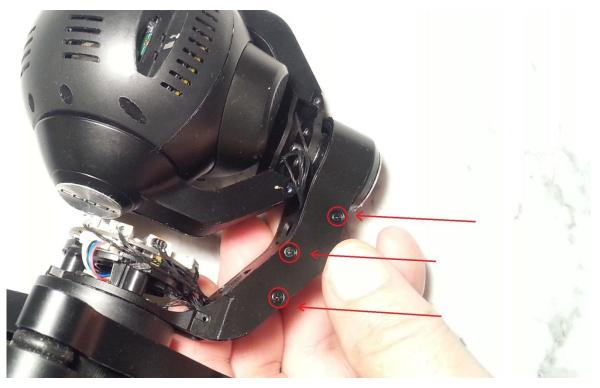
33. Install the lower wire cover and both screws:
