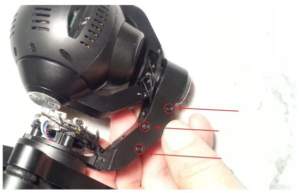
12. Use fingernails or thin plastic to remove the label over the Roll motor:
