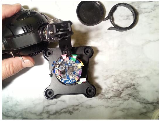
13). Remove the three gimbal board mounting screws:
