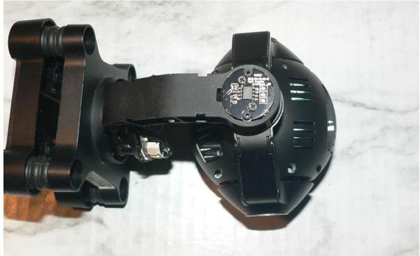
30). Install the rear arm cover and :rear screws
