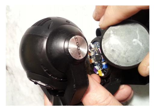
3. Remove the two screws (one on each side) holding the Gimbal Board Enclosure to the rear arm:
