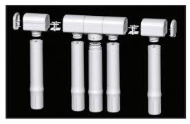
This drawing illustrates some of the customizable filter connection options the HERO-375Plus has to offer. Additional filter(s) may be added on to either side of standard unit.
