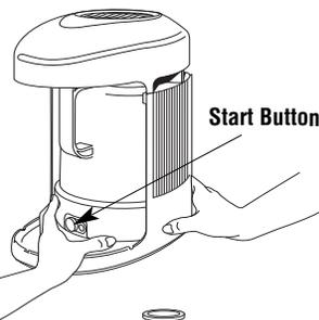
**CAUTION:** To prevent personal injury or property damage the boiling chamber must be fully engaged prior to start-up.
