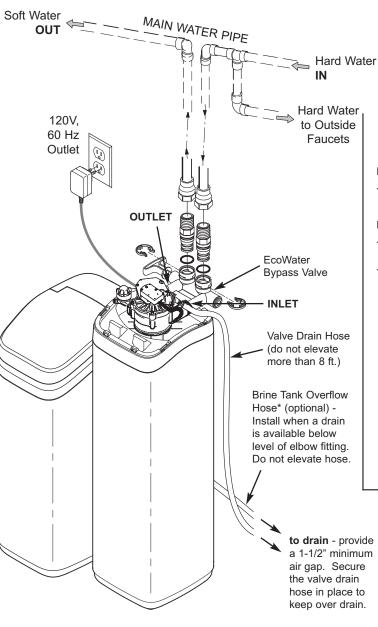
\*Do not connect the water softener valve drain hose to the brine tank overflow hose.
