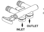
Turn the bypass valve downward if connecting to floor level plumbing
