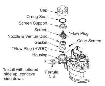
IMPORTANT: Be sure small hole in the gasket is centered directly over the small hole in the nozzle & venturi housing. Be sure the numbers are facing up
