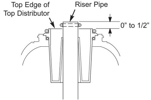
**Note:** Resin tank height can vary somewhat within manufacturing tolerance. So that the bottom distributor riser pipe has proper clearance with inside valve porting, check for the correct length, as shown above. Cut the riser pipe if needed to adjust the length. Be sure to remove burrs and sharp edges.
