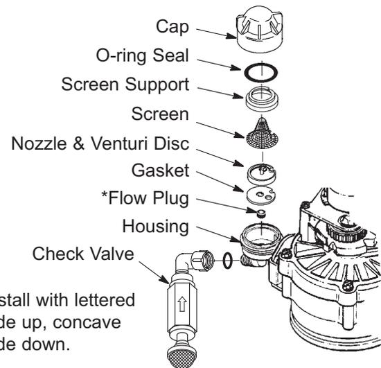
**IMPORTANT:** Be sure small hole in the gasket is centered directly over the small hole in the nozzle & venturi housing. Be sure the numbers are facing up
