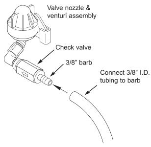
Place other end of tube in hydrogen peroxide solution
