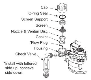
IMPORTANT: Be sure small hole in the gasket is centered directly over the small hole in the nozzle & venturi housing. Be sure the numbers are facing up
