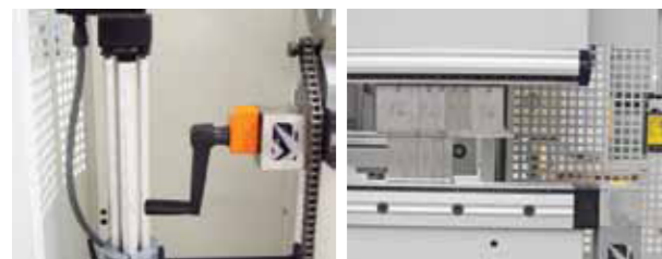
▶ Original WILA 'Opposing wave' Motorized Crowning System Optional *(Standard according size of machine )
