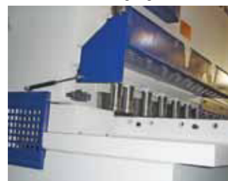
▶ Front Finger Protection Open able 1000 mm
