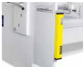
▶ Rear Protection Light Beams
