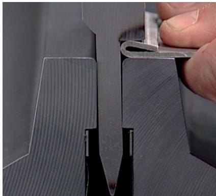
Pre-bend and flattening in the same tool.
