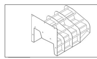
Gutter forms supported in dimensions ranging from 24 inches high (610mm) to 30 inches wide (762mm)
