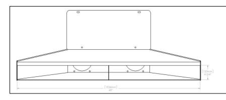
Sidewalk forms supported in dimensions up to 6 feet wide (1.828 meters) to a depth up to 12 inches ( 304mm)
