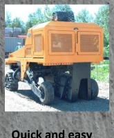
Quick and easy mold change from curb to gutter or to sidewalk
