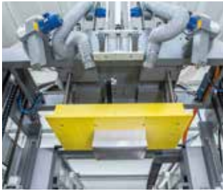
Upper mould plate (for pressure forming) Piano stampo superiore (per pressione formatura)
