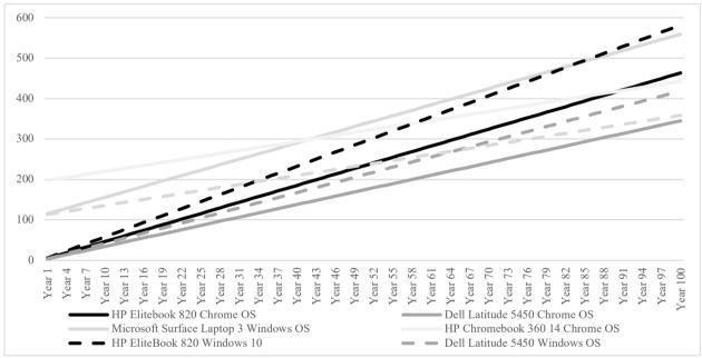
Figure 1. Cumulative greenhouse gas emissions (kgCO<sub>2</sub>e) generated by end user computing devices
