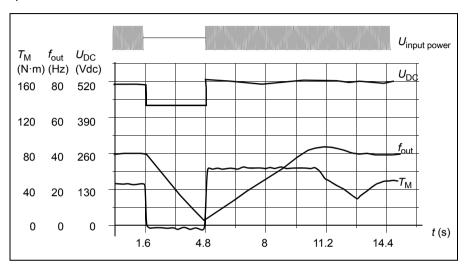
$U_{\rm DC}$  = Intermediate circuit voltage of the drive,  $f_{\rm out}$  = Output frequency of the drive,  $T_{\rm M}$  = Motor torque
