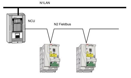
The following diagram shows the drives' integration to the Johnson Controls Metasys Companion system.
