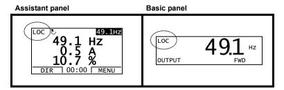
The control panel always overrides the external control signal sources when used in local mode.
