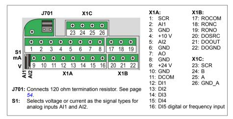
WARNING! All ELV (Extra Low Voltage) circuits connected to the drive must be used within a zone of equipotential bonding, in other words, within a zone where all simultaneously accessible conductive parts are electrically connected to prevent hazardous voltages appearing between them. This is accomplished by a proper factory grounding.
