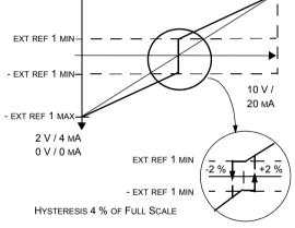
WARNING! Because the low end of the reference range commands full reverse operation, do not use 0 V as the lower end of the reference range. Doing so means that if the control signal is lost (which is a 0 V input) the result is full reverse operation. Instead, use the following set-up so that loss of the analog input triggers a fault, stopping the drive:
