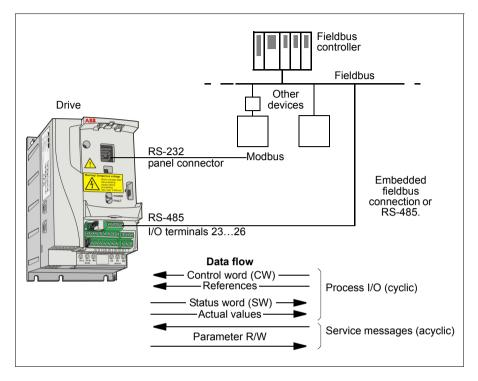
The drive can be set to receive all of its control information through the fieldbus interface, or the control can be distributed between the fieldbus interface and other available sources, for example, digital and analog inputs.
