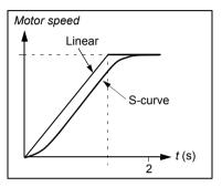
S-curve: Ideal for conveyors carrying fragile loads, or other applications where a smooth transition is required when changing the speed.
