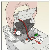
6. Disconnect the fan cable. The figure below on the right shows the location of the fan cable connector in frame size R2. The inside views in different frame sizes are not identical, but the fan cable connector is always on the control board that is against the front of the drive.
