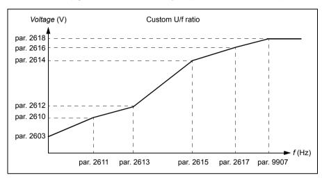
**Note:** The voltage and the frequency points of the U/f curve must fulfill the following requirements:
