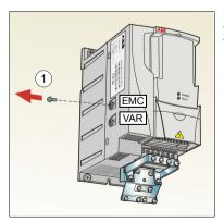
Note: In frame size R4 the EMC screw is located to the right of terminal W2.
