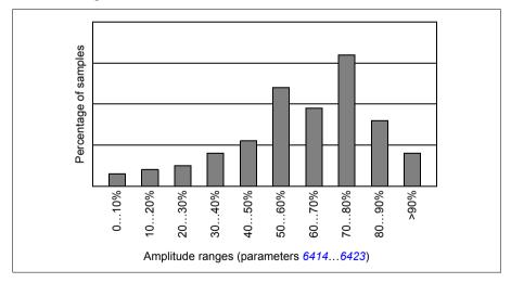
Amplitude logger 1 (AL1) is fixed to monitor output current, and it cannot be reset. With amplitude logger 1, 100% corresponds to the nominal output current of the drive  $(I_{2N}).$
