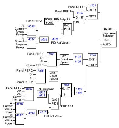
**Note:** To activate and use the PID controller, parameter 1106 REF2 SELECT must be set to value 19.
