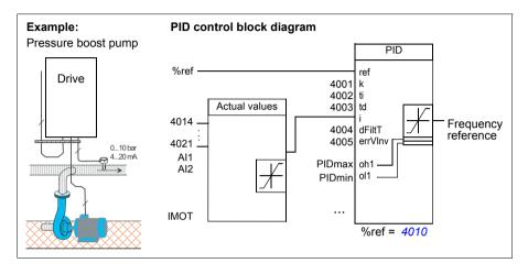
The following figure presents the speed/scalar control block diagram for process controller PID1.
