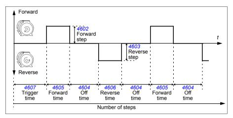
The pump cleaning cycle can be activated at start-up, with a user-defined period, with a selectable digital input or by the Supervision function (for example triggered by the motor input current).
