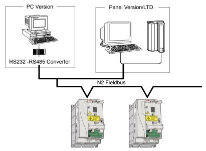
On the N2 fieldbus each ACS320 drive can be accessed by the full complement of Metasys FMS features, including Change-of-State (COS) monitoring, alarm notification, scheduling, trend, and totalization.
