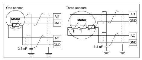
WARNING! According to IEC 664, the connection of the motor temperature sensor requires double or reinforced insulation between motor live parts and the sensor. Reinforced insulation entails a clearance and creepage distance of 8 mm (400/500 V AC equipment).
