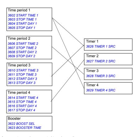
A parameter can be connected to only one timer.
