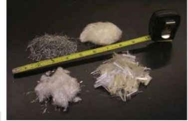
Fig. 5.2.2—Examples of fibers used to control shrinkage cracking.
